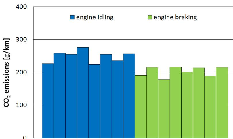
Fig. 6. The road emission of CO<sub>2</sub> determined for the analysed driving techniques
