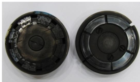
Fig. 2. Example of model friction pair used in IL-68 tests (right friction material samples, left cast iron counter sample)
