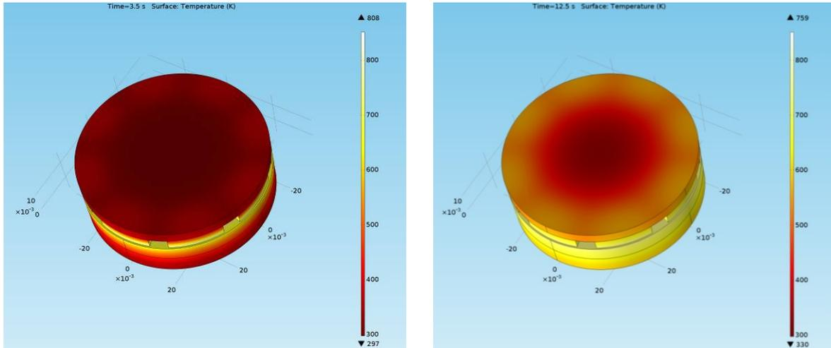
Fig. 4. Sample frames of FEM model temperature calculations
