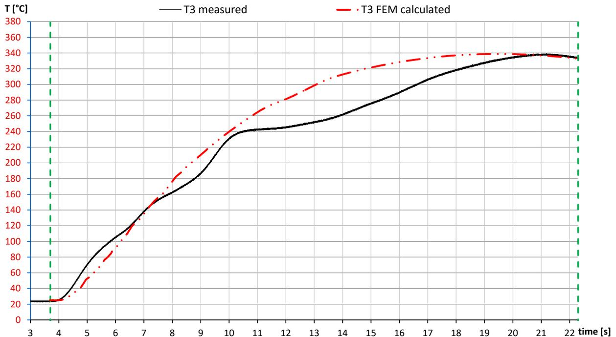
Fig. 5. Comparison between curves of measured and FEM calculated temperatures
