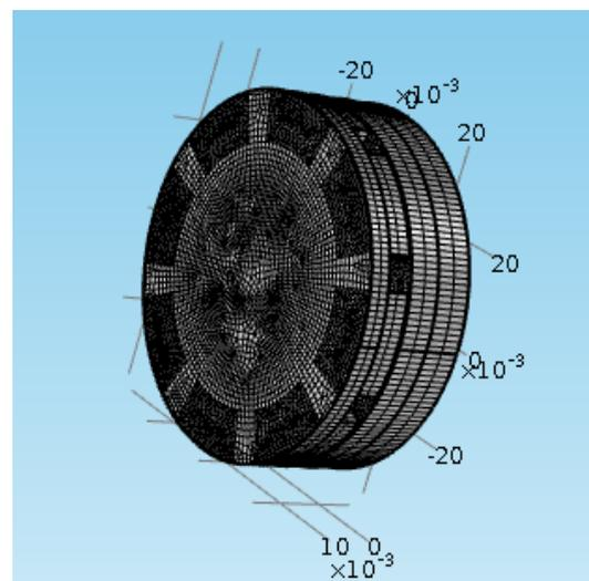
Fig. 4. Meshed FEM model
