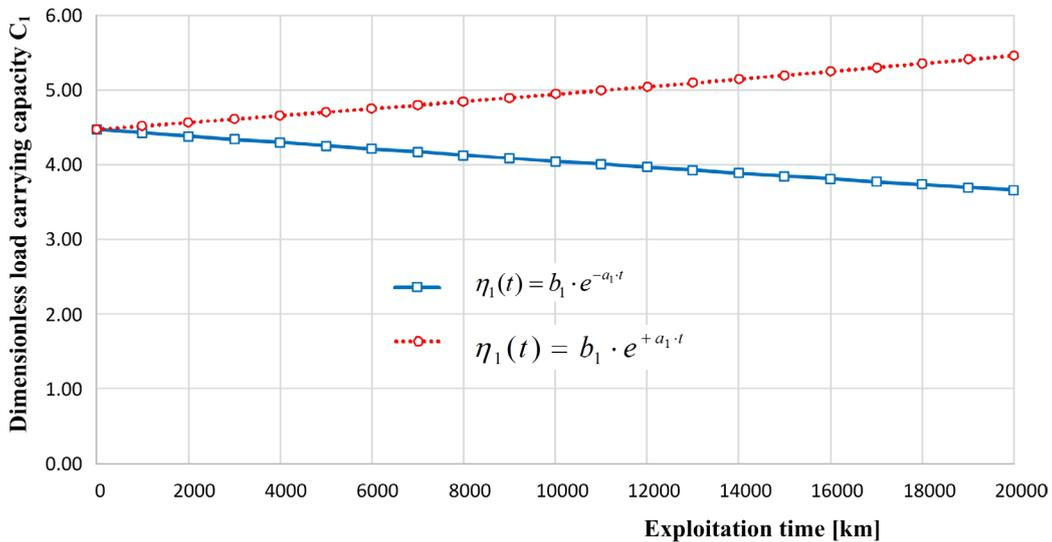
Fig. 4. Dimensionless values of the carrying capacity load for the decreasing and increasing dynamic viscosity in exploitation time:  $\eta_1(t) = b_1 \cdot e^{-a_1 t}$  and  $\eta_1(t) = b_1 \cdot e^{+a_1 t}$
