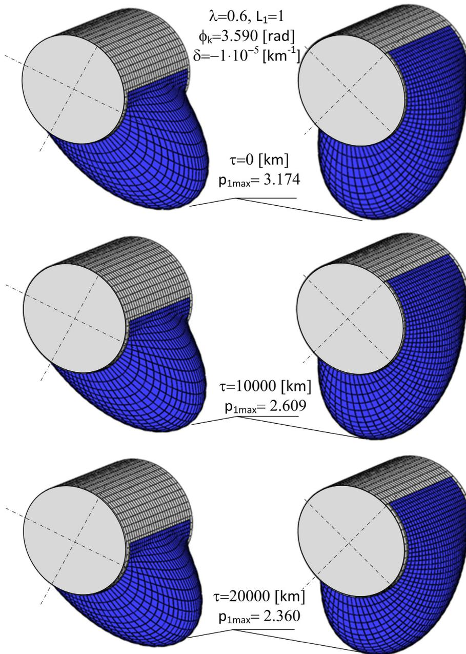
Fig. 1. The dimensionless pressure distributions  $p_1$  in cylindrical sliding journal bearings for  $\eta_1(t) = b_1 \cdot e^{-a_1 t}$
