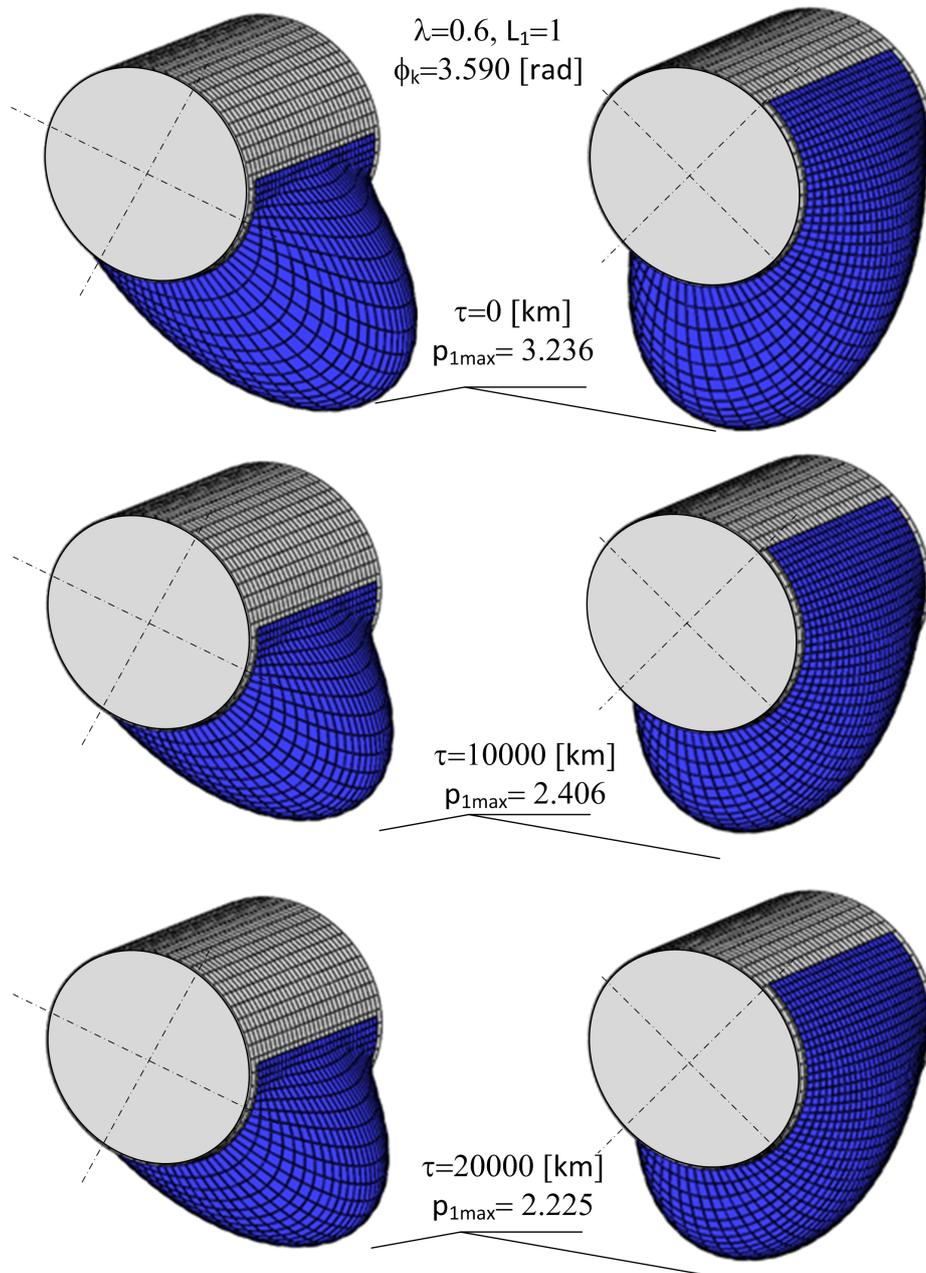
Fig. 2. The dimensionless pressure distributions  $p_1$  in cylindrical sliding journal bearings for  $\eta_1(t) = a \cdot t^6 - b \cdot t^5 + c \cdot t^4 - d \cdot t^3 + e \cdot t^2 - f \cdot t + 1$
