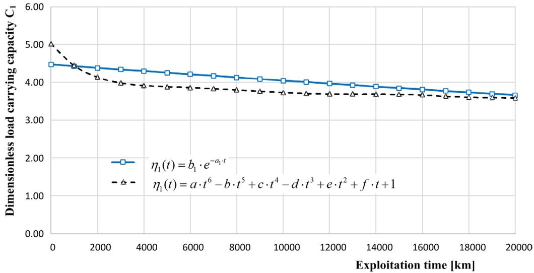
Fig. 3. Dimensionless vaules of the carrying capacity load for two models of viscosity changes in exploitation time:  $\eta_1(t) = b_1 \cdot e^{-a_1 t}$  and  $\eta_1(t) = a \cdot t^6 - b \cdot t^5 + c \cdot t^4 - d \cdot t^3 + e \cdot t^2 - f \cdot t + 1$
