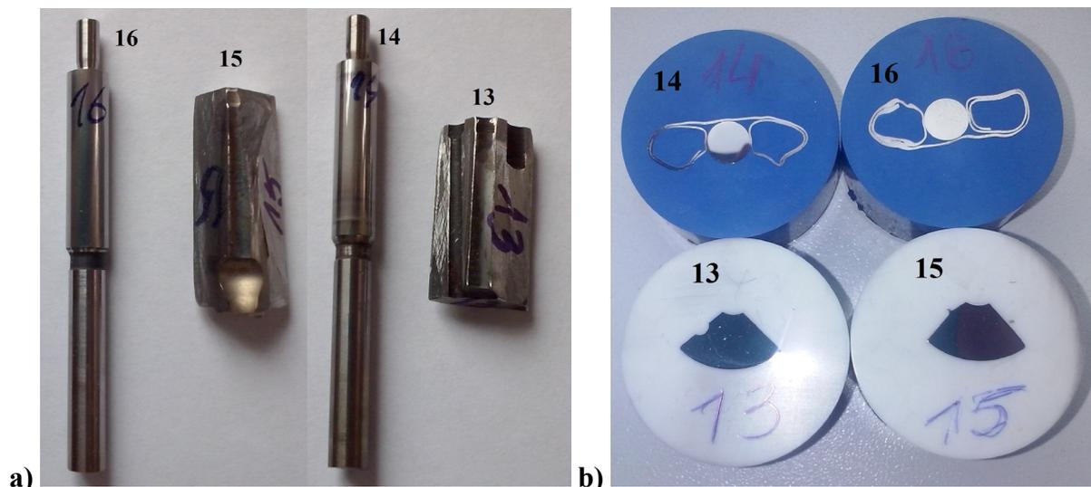
Fig. 1. The investigated parts of DLLA 160 S 1305 injector: a) the view of the injector needle and body, b) the corresponding prepared samples; 16 – new injector tip needle, 14 – used injector tip needle, 15 – new injector tip body, 13 – used injector tip body
