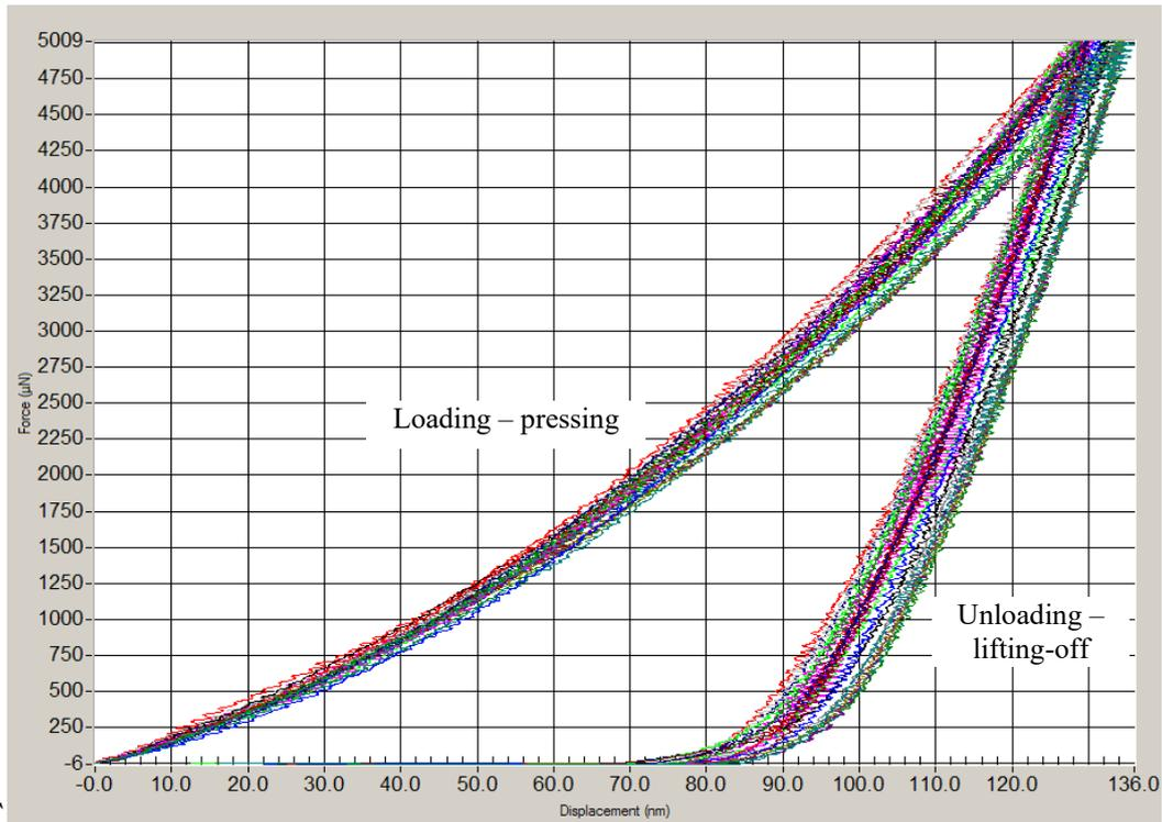
Fig. 3. Exemplary diagram showing the surface deformation during loading and unloading – sample of the injector tip body (used)
