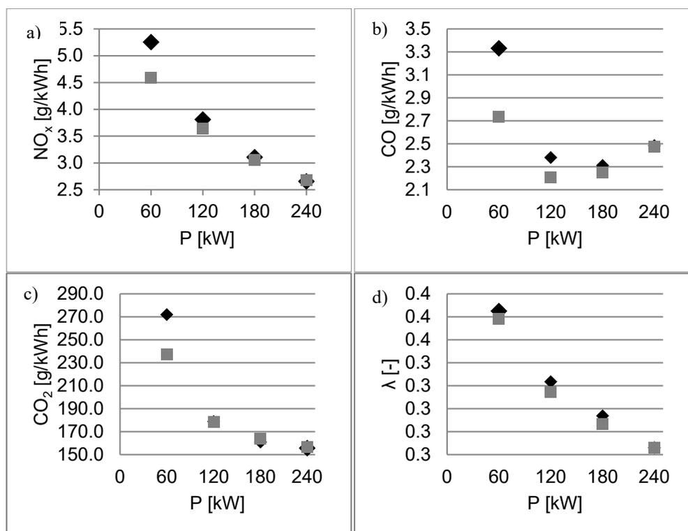
Fig. 3. The results of the a) NO<sub>x</sub>, b) CO, c) CO<sub>2</sub> emissions and d) λ for all considered loads and observations: ◆ – The engine assumed as operated without malfunctions, ■ – throttling of the exhaust gas duct
