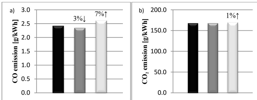
Fig. 2. The values of the total weighted CO,  $CO_2$  emissions: ■ – engine assumed as operated without malfunctions, ■ – throttling of the exhaust gas duct, ■ – throttling of the intake air duct
