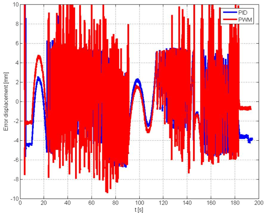
Fig. 7. Comparison of displacement errors for the displacement piston rod for boom mechanism control with PID and PWM controller
