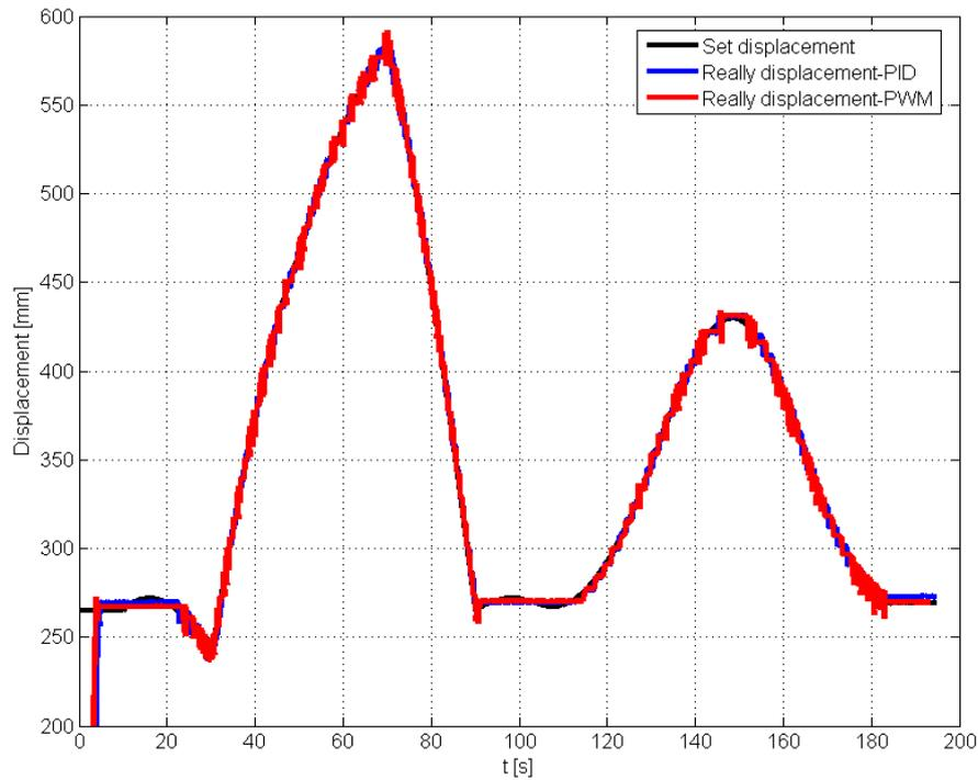
Fig. 5. Comparison of the displacement piston rod for boom mechanism control with PID controller and PWM controller
