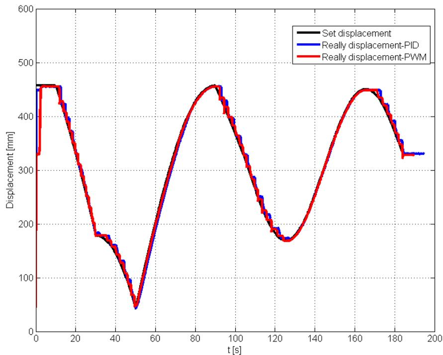
Fig. 6. Comparison of the displacement piston rod for arm mechanism control with PID controller and PWM controller
