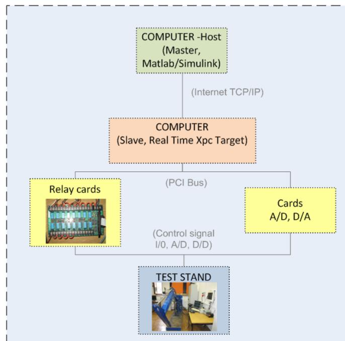
*Fig. 3. Scheme of control system for test stand*
