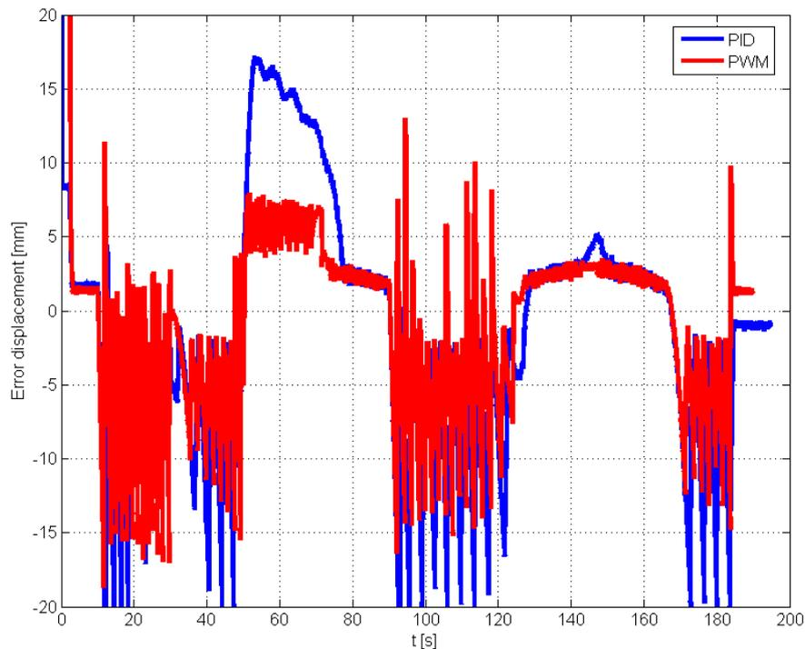
Fig. 8. Comparison of displacement errors for the displacement piston rod for arm mechanism control with PID and PWM controller
