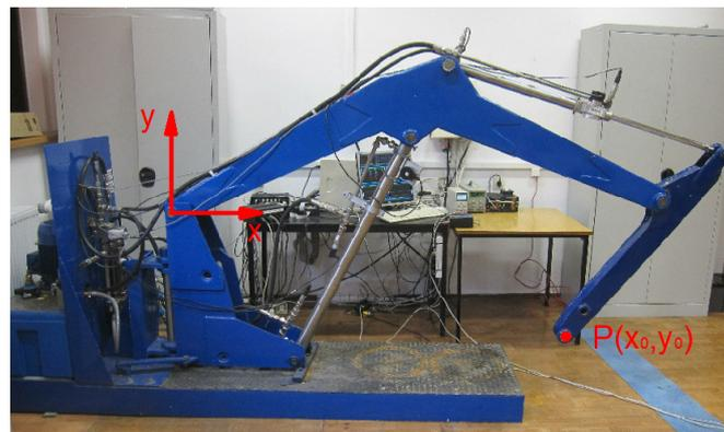
Fig. 1. Scheme of test stand and placement of Cartesian system and the location of the point P
