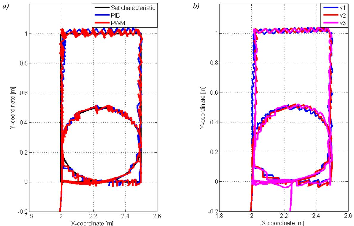
Fig. 9. Characteristics of discrepancies reference signal from a real signal for: two systems of controller (a), three different velocity of mechanisms (b)
