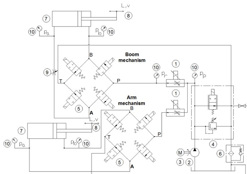
Fig. 2. Diagram of the hydraulic system
