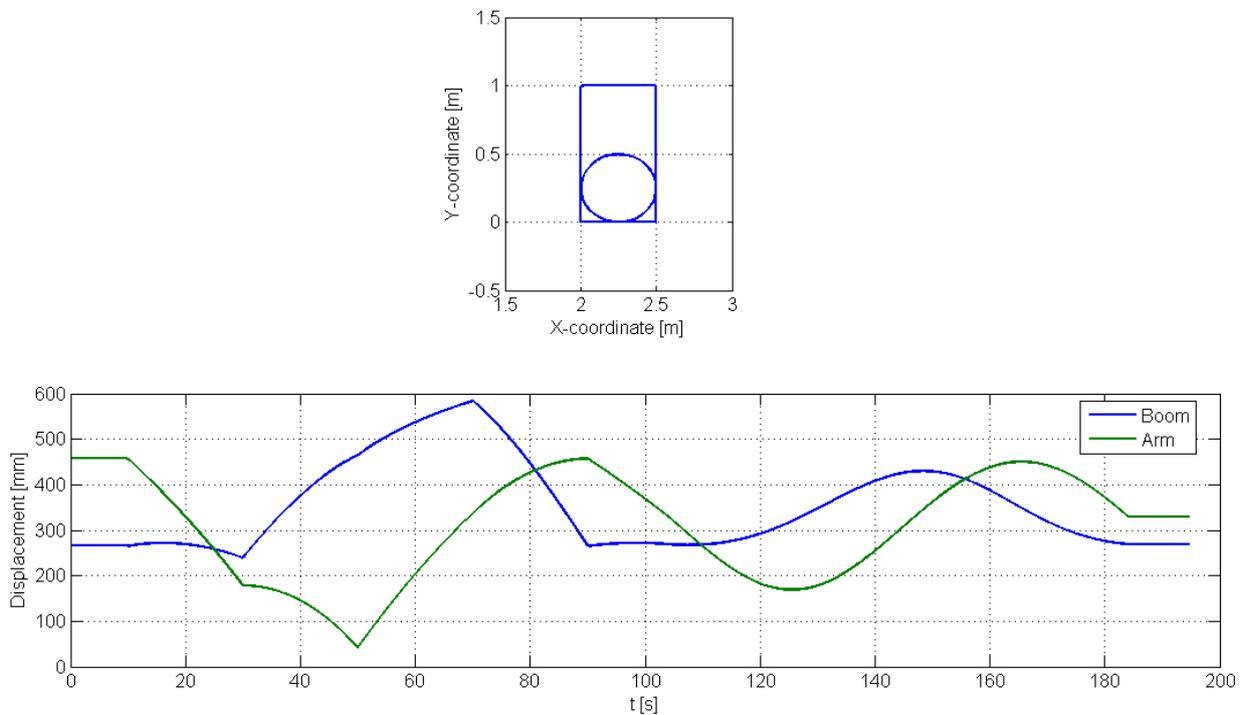
Fig. 4. Standardized signal with the displacement of boom cylinder and arm
