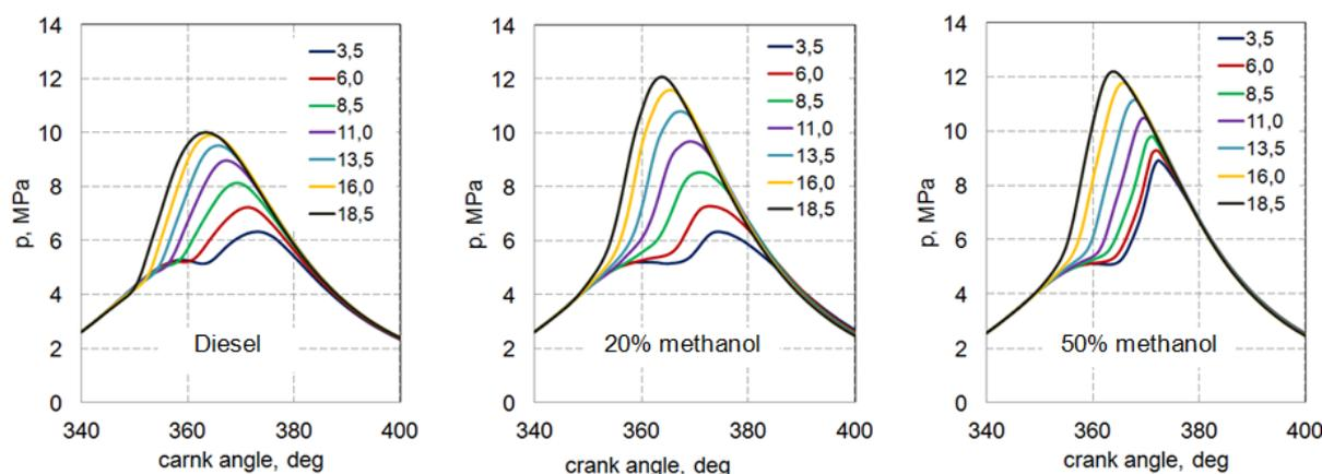
Fig. 4. The courses of the combustion pressure in a diesel and dual fuel engine
