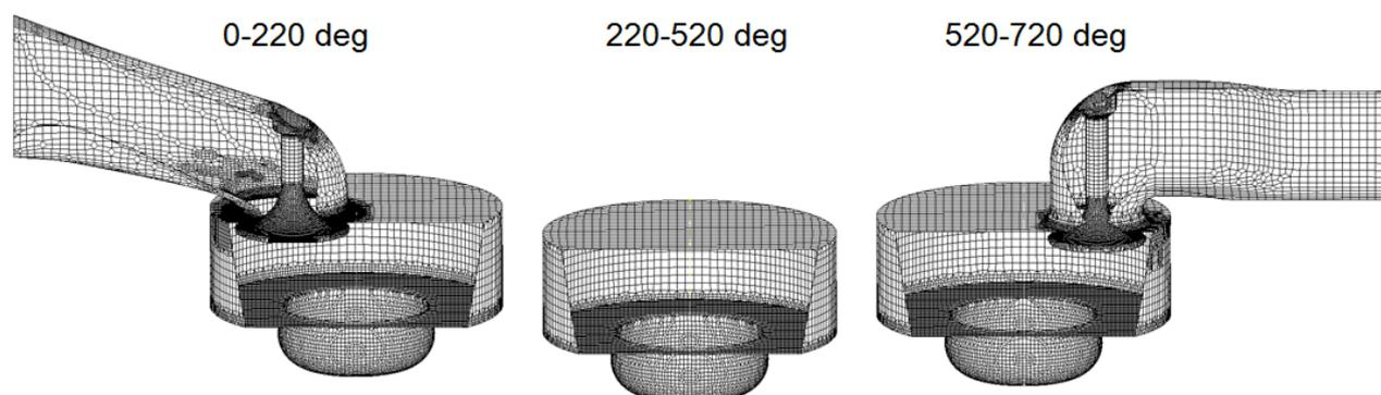
Fig. 1. The computational mesh of engine
