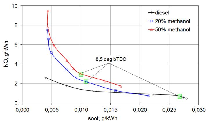
Fig. 5. The interdependence of NO and soot emission in a dual fuel engine
