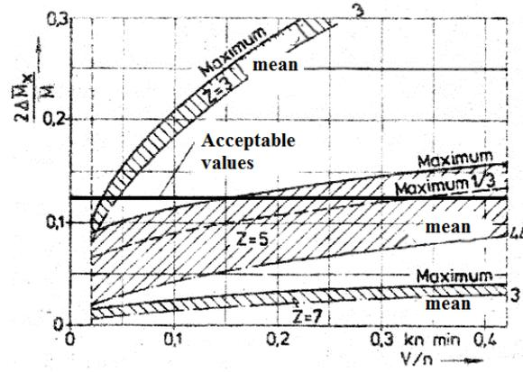
Fig. 4. Double mean values, maximum and mean values of the three highest dimensionless amplitudes of vibrating moment for the propeller of blade numbers 3, 5 and 7 in different work conditions [1]
