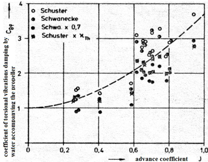
Fig. 2. Coefficient of torsional vibrations damping by the mass of water accompanying the propeller in the function of advance coefficient with calculations according to Schuster and Schwanecke [1]
