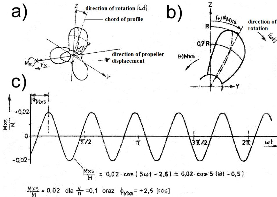
Fig. 3. Course of the moment caused by torsional vibrations of 5 blade propeller; a) arrangement of coordinates describing motion of the propeller; b) plane of torsional vibrations; c) course of rotation moment vibrations
