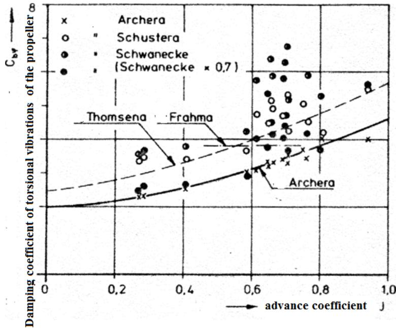
Fig. 1. Coefficient of torsional vibrations damping of the propeller and function of advance coefficient with plotted values received from different formulas [1]
