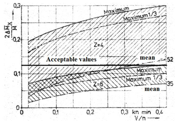
Fig. 5. Double means values, the highest and mean values of the three highest dimensionless amplitudes of vibrating moment for the propeller of blade numbers 4 and 6 in different work conditions [1]
