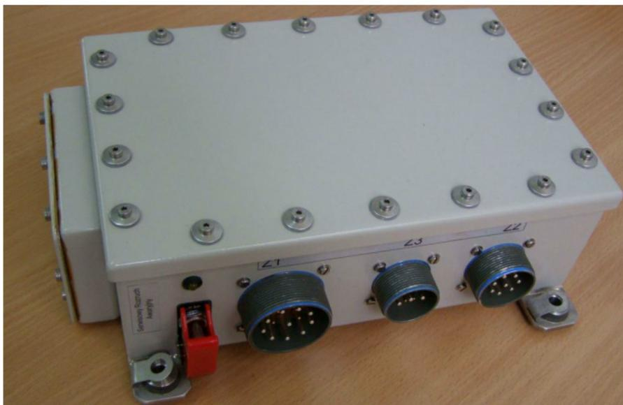
*Fig. 8. MUR-2 Microprocessor starting device*
