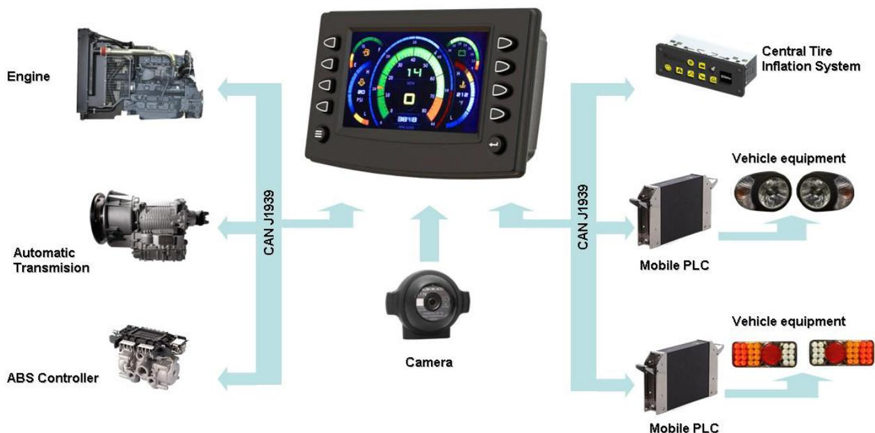
Fig. 6. Visualisation of the DK-15 Dashboard solution
