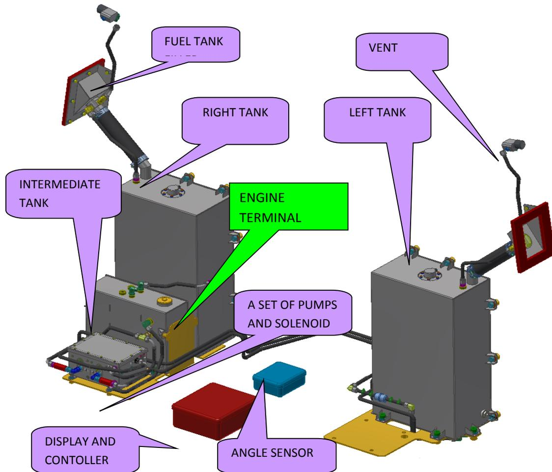
*Fig. 10. Diagram of the fuel system*
