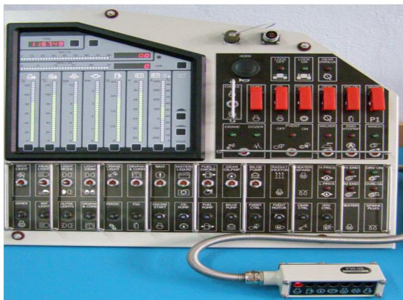
Fig. 3. The PK-08 Control Panel with the PW-08 version up to the WZT-3
