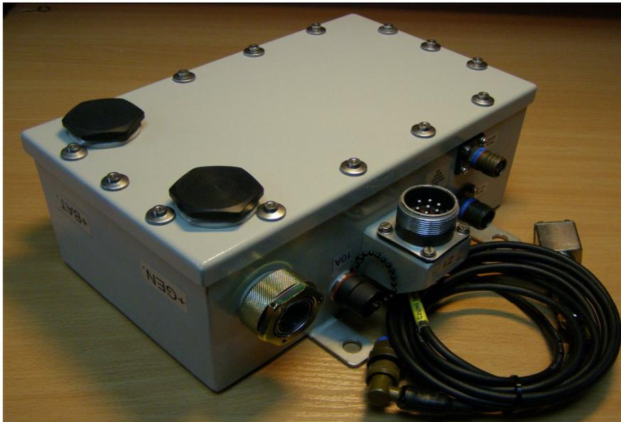
*Fig. 7. Voltage Regulator RN-10U2*
