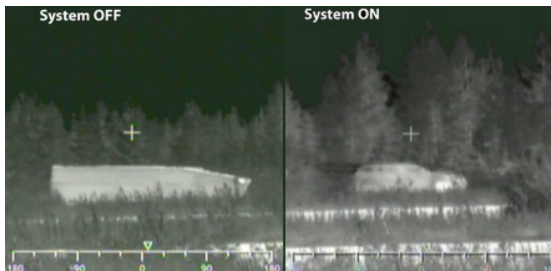
Fig. 3. The armoured vehicle fitted with 'Adaptive' infrared side panels, switched off (left), and on to simulate a large car (right)
