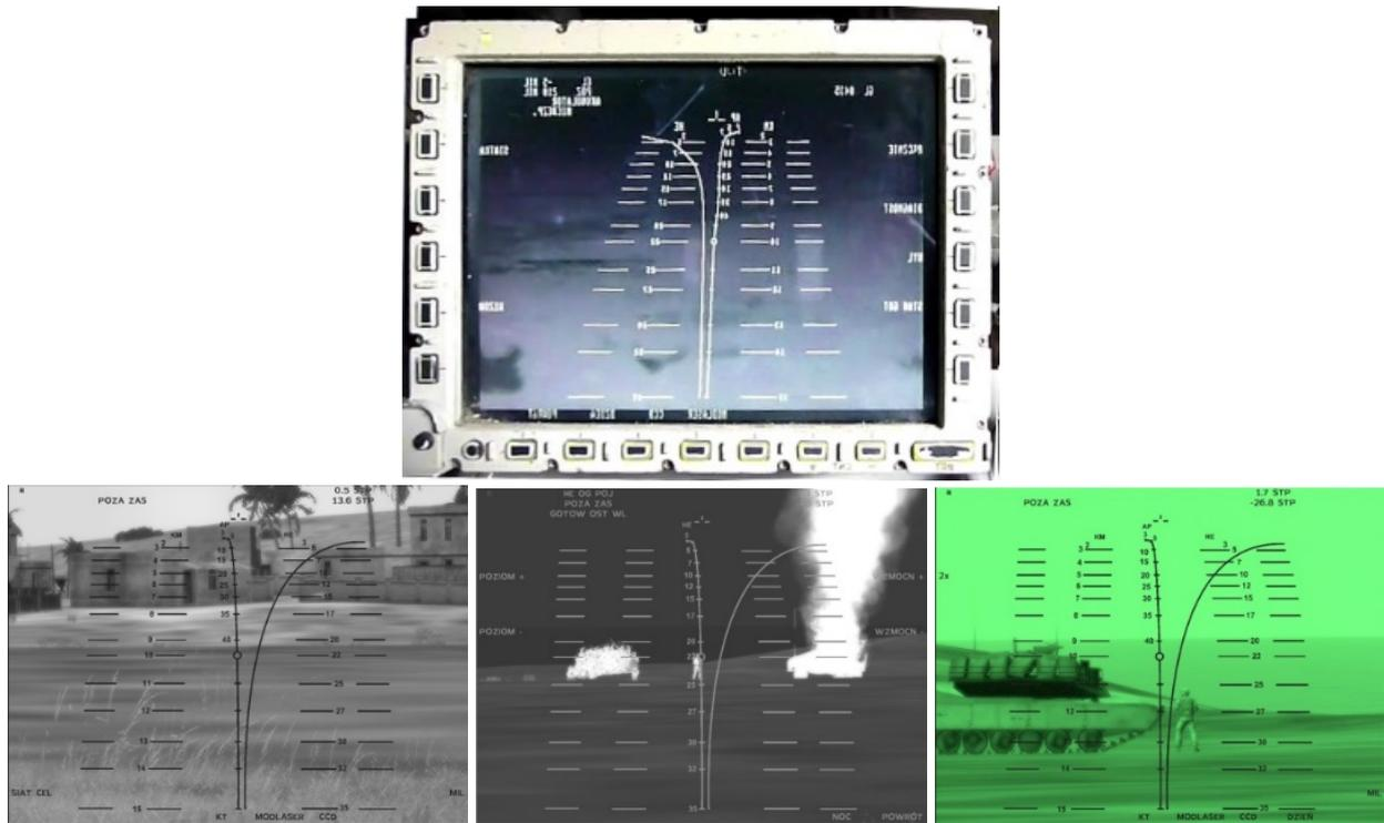
Fig. 5. Examples of simulated imaging on the monitors of the Fire Control System in the SK1-Pluton simulator (real monitor and virtual imaging [6])
