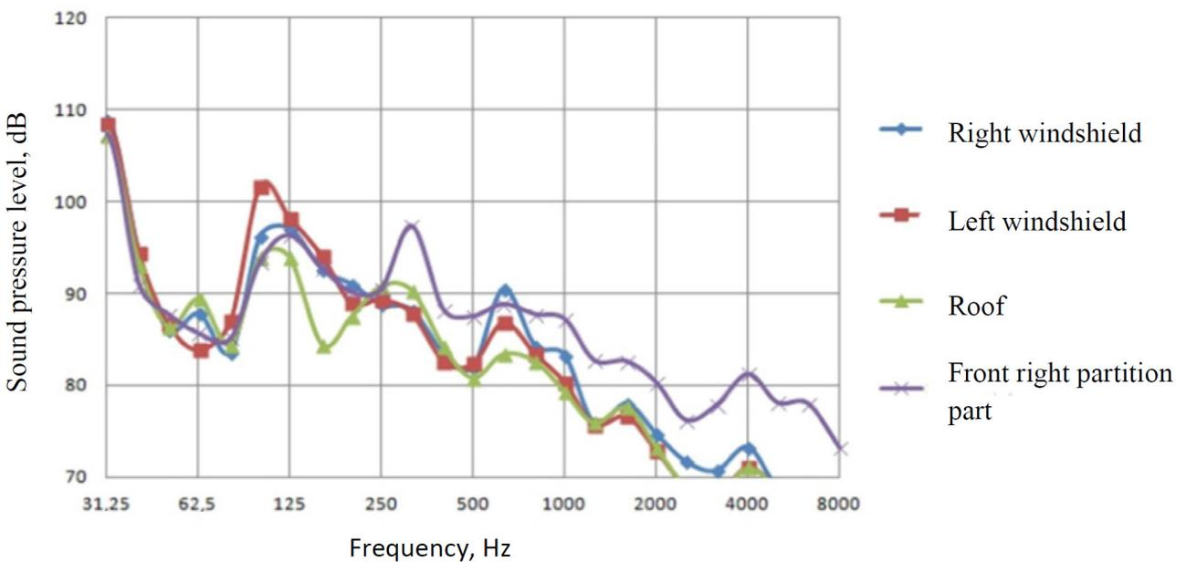
Fig.3. Noise from cabin panels during tractor without aggregate motion
