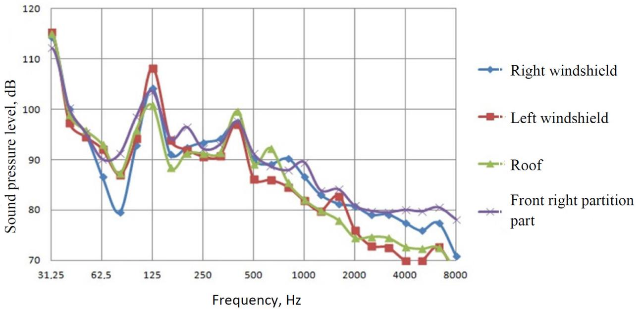
Fig.2. Noise from cabin panels during tractor with seeding aggregate motion
