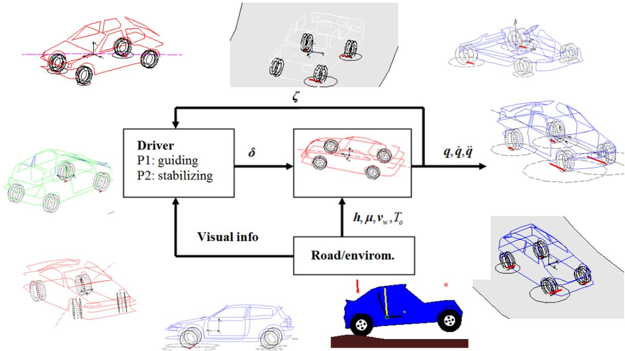
Fig. 2. „miMa” model of driver-vehicle-road system for optimization tasks in motorsport
