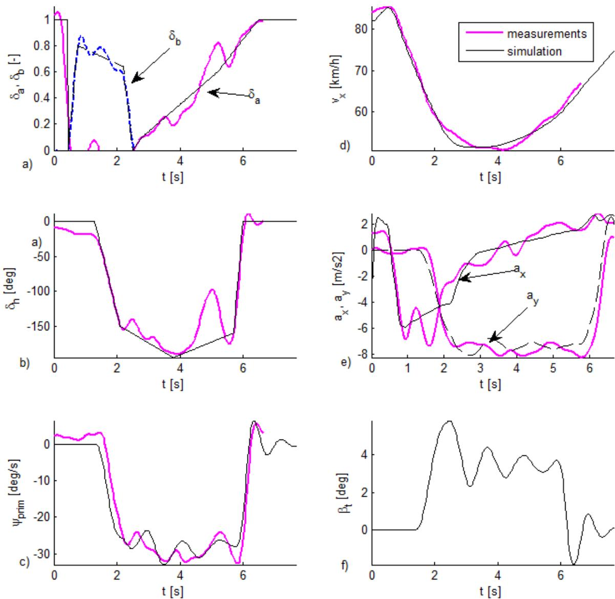
Fig. 4. Comparison of measured and simulated time profiles of RH corner maneuver with LADA VFTS
