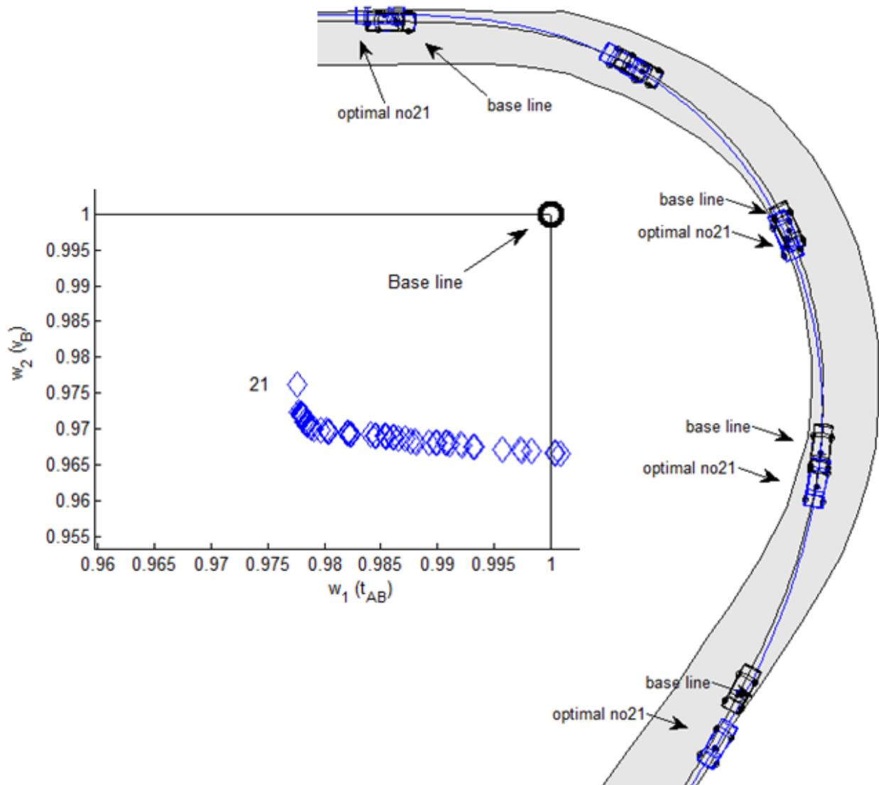
Fig. 5. Pareto-optimal results (left) and (right) comparison of base line and optimal no21 trajectories of Lada VFTS
