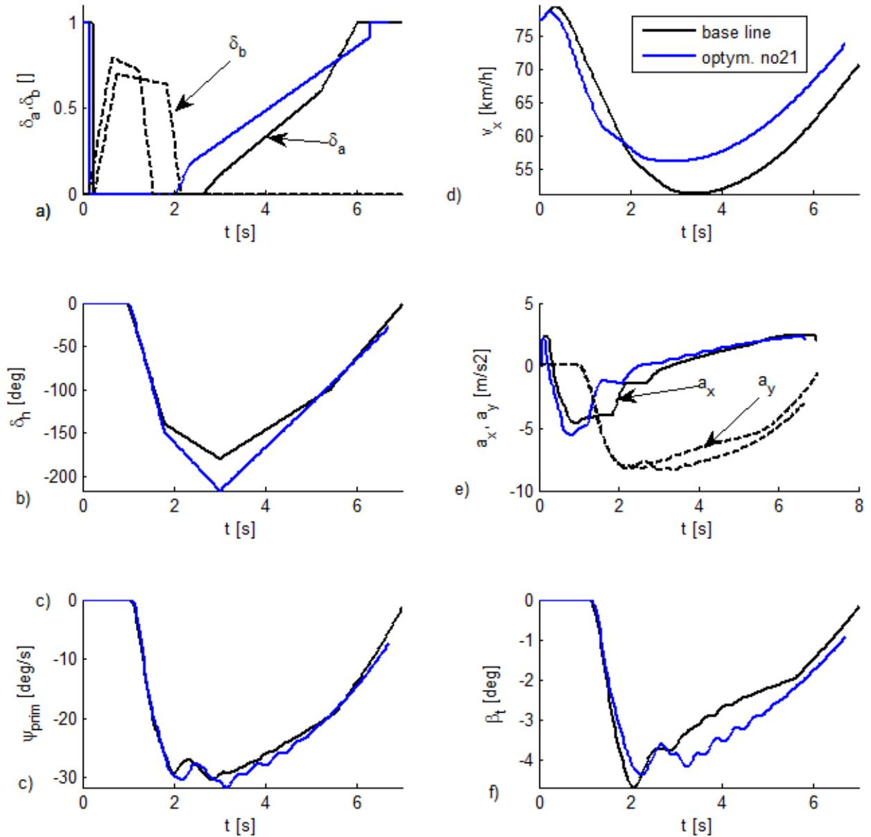
Fig. 6. Comparison of time profiles of RH corner maneuver with LADA VFTS for base line setup and optimal (no21) driver actions
