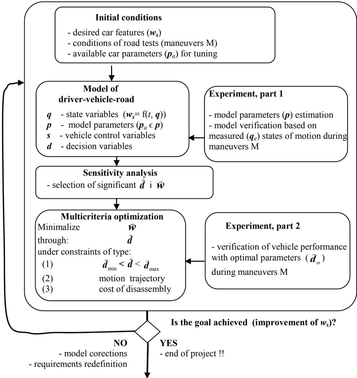
Fig. 1. “miMa” algorithm for a car performance increase through optimization of its computer model
