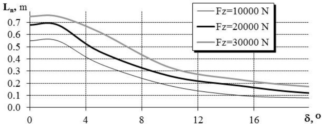
Fig. 2. Changes in the relaxation length  $L_n$  of typical truck tire due wheel normal  $F_z$  load and side cornering angle  $\delta$
