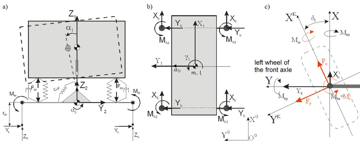
Fig. 4. The scheme of the vehicle physical model; a) front view; b) top view; c) system of forces and torques transmitted by the wheel from the road surface to the vehicle chassis, shown as the example of the left front vehicle wheel
