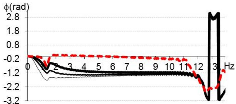
Fig. 8. Dynamic characteristics of the vehicle model determined for the lateral acceleration  $a_{1y}$  in the centre of the vehicle body mass
