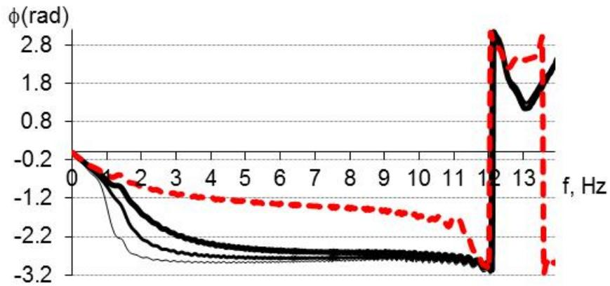
Fig. 7. Dynamic characteristics of the vehicle model determined for the yaw angular velocity  $\dot{\gamma}_1$  of the vehicle body
