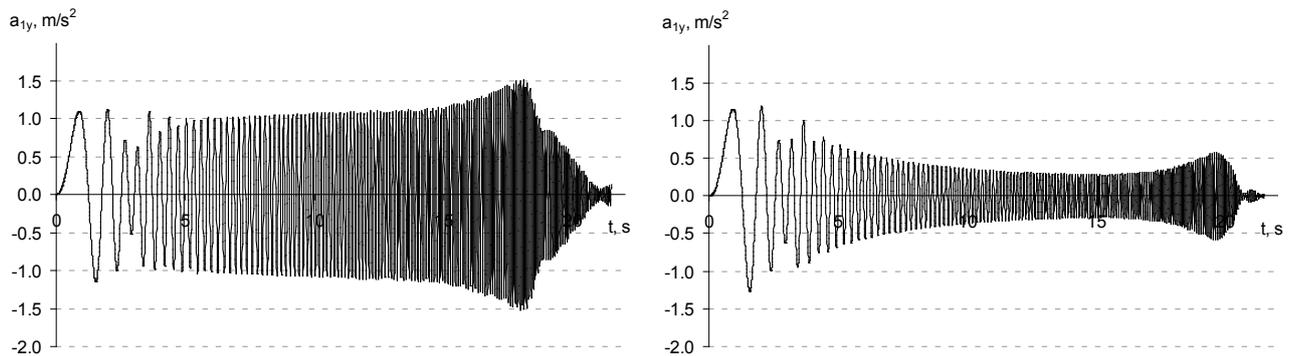
Fig. 6. Preliminary simulation results - time courses; a) steered wheels turning angle - signal forcing the vehicle dynamics model; b) vehicle response - yaw angular velocity  $\dot{\gamma}_1$  of the vehicle body; c) vehicle response - lateral acceleration  $a_{1y}$  in the centre of the vehicle body mass
