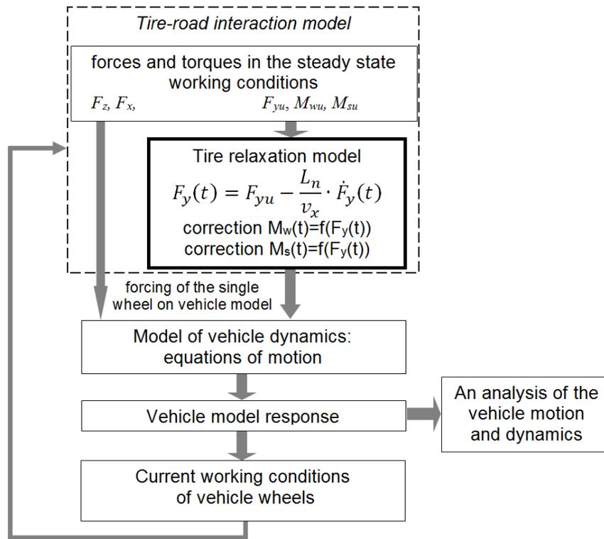
Fig. 5. Calculations scheme of vehicle dynamics model – connections between the tire-road interaction model with the tire relaxation model and vehicle dynamics model
