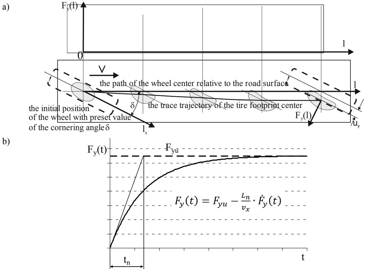
Fig. 1. Model course of the tire relaxation process because of a step-change in the wheel side cornering angle  $\delta$ ; a) Increase of the side reaction force  $F_y$  as a function of the distance travelled by the wheel in the quasi-static conditions; b) The IPG-Tire model - the course of the function and the model equation
