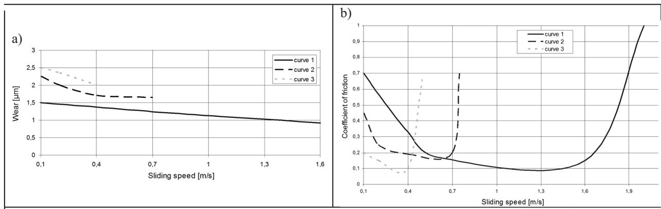
Fig. 4. Dependence of wear (a) and the coefficient of friction (b) on the sliding speed for the matching of the friction assembly of the ball plunger face made of steel HWG with the swivel disk made of steel EI-928; 1-pressure  $P_{os} = 100$  N, 2- pressure  $P_{os} = 1400$  N, 3-pressure  $P_{os} = 600$  N
