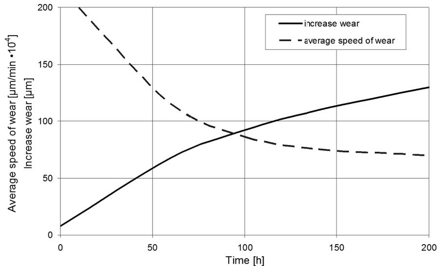
Fig. 8. Change of the wear of the ball plunger face in the pump NP-34, depending on the working time (one of the result achieved during the stand tests)
