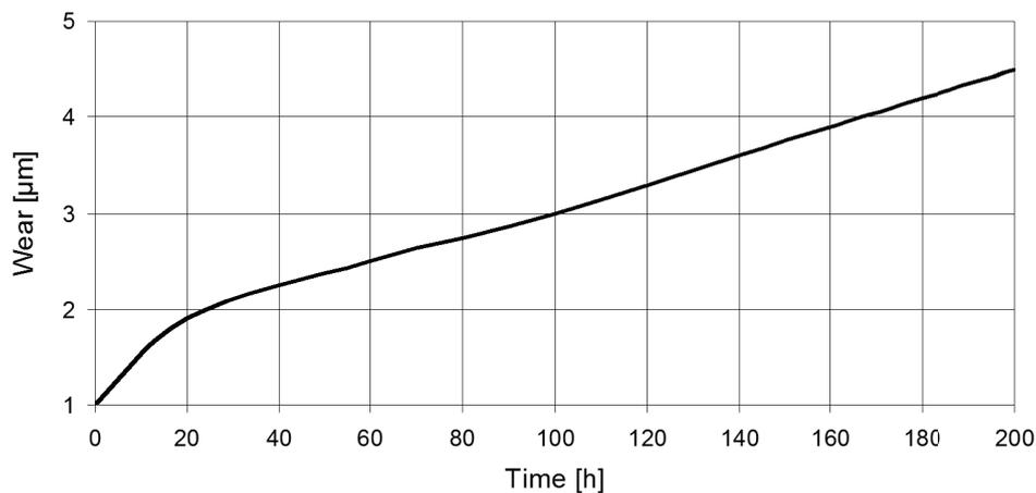
Fig. 9. Change of the wear of the working surface of the steering swivel disk in the pump NP-34, depending on the working time (one of the result achieved during the station tests)
