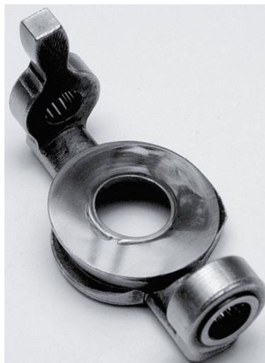
*Fig. 3. Working surface of the steering swivel disk in the hydraulic plunger pump*
