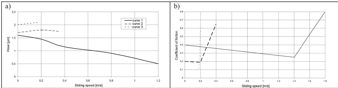
Fig. 6. Dependence of wear on the sliding speed for the matching of the friction assembly of the ball plunger face made of steel 18HNWA with the swivel disk made of steel EI-928; 1- pressure  $P_{os} = 100$  N, 2- pressure  $P_{os} = 600$  N, 3- pressure  $P_{os} = 1400$  N
