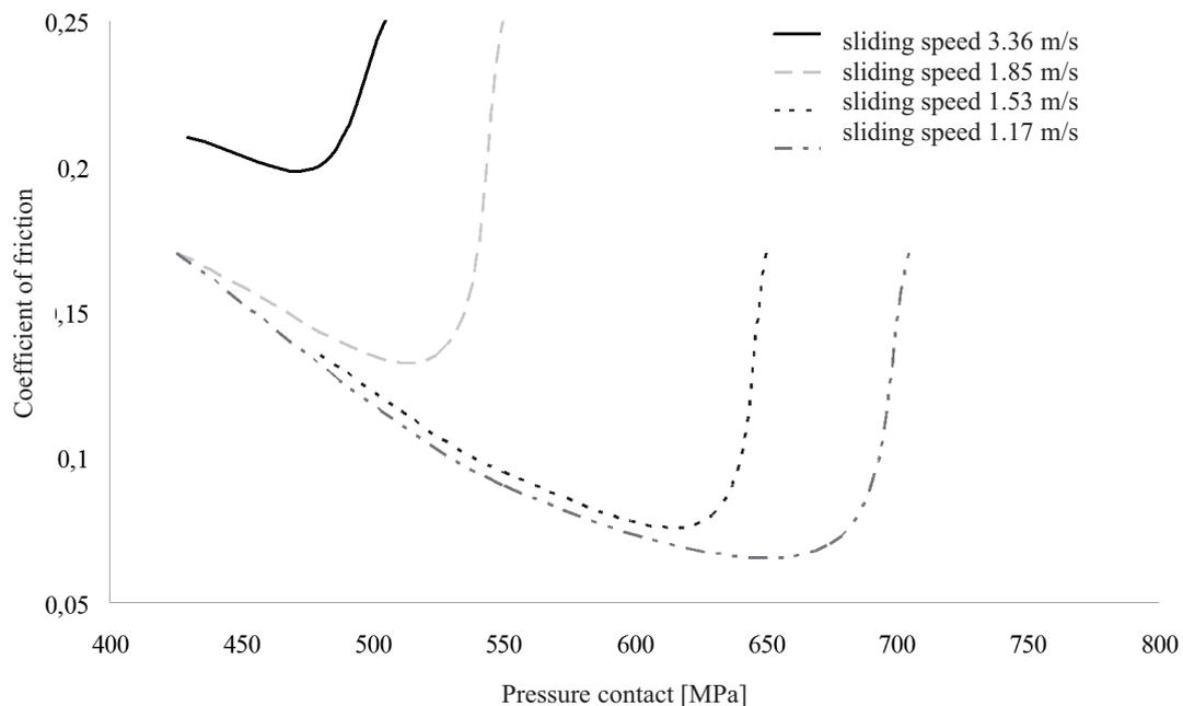
Fig. 7. Dependence of the coefficient of friction in the plunger assembly on the contact pressure at different sliding speeds
