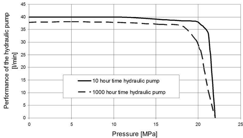
*Fig. 10. Dependence of the efficiency of the hydraulic pump on pressure*
