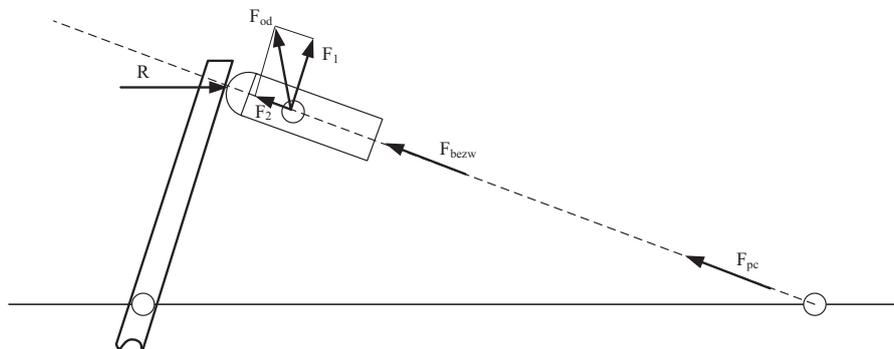
Fig. 1. Diagram of loading the hydraulic plunger assembly:  $F_{pc}$  – pressure force of the working liquid;  $F_{bezw}$  – inertial force by relative movement;  $F_{od}$  – centrifugal force;  $R$  – reaction force of the plunger face;  $F_1$  and  $F_2$  – components of the centrifugal force
