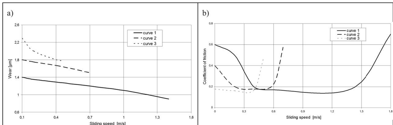
Fig. 5. Dependence of wear (a) and the coefficient of friction (b) on the sliding speed for the matching of the friction assembly of the ball plunger face made of steel 12HN3A with the swivel disk made of steel EI-928; 1-pressure  $P_{os} = 100$  N, 2- pressure  $P_{os} = 600$  N, 3- pressure  $P_{os} = 1400$  N
