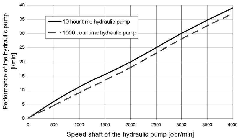
*Fig. 11. Dependence of the efficiency of the hydraulic pump on the rotational speed of its drive shaft*
