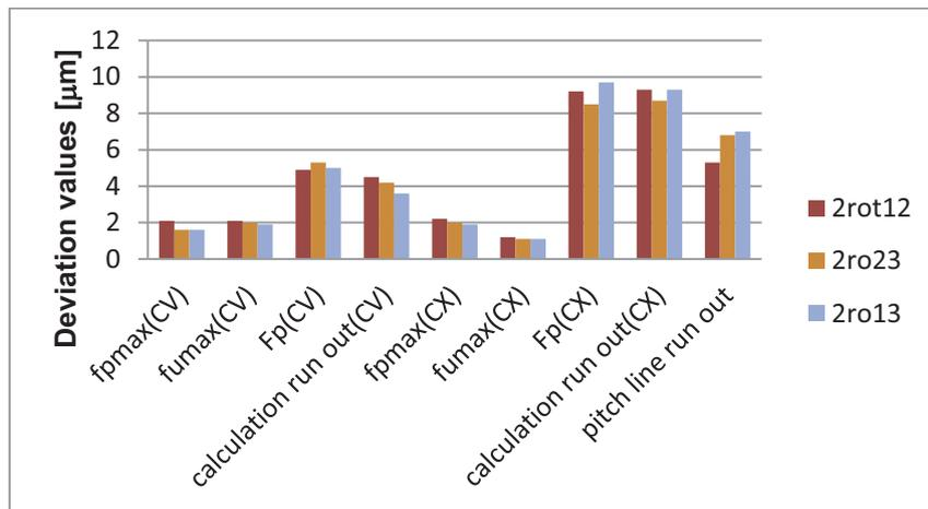
Fig. 4. Performance deviation values (*fpmax*, *fumax*, *Fp*, run out calculation, pitch line run-out) obtained from the measurement of a bevel gear with circular pitch line whose fixation error compensation is based on 2 radial run-out measurements of the reference surface
