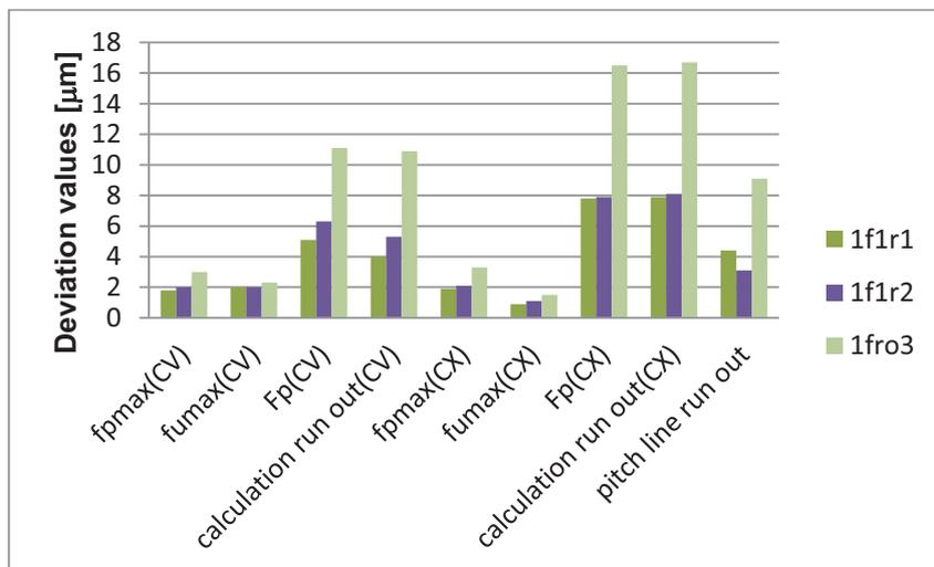
Fig. 5. Performance deviation values (*fpmax*, *fumax*, *Fp*, run out calculation, pitch line run-out) obtained from the measurement of a bevel gear with circular pitch line, whose fixation error compensation is based on 1 axial run-out measurement and 1 radial run-out measurements of the reference surface
