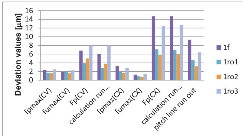
Fig. 6. Performance deviation values (fpmax, fumax, Fp, run out calculation, pitch line run-out) obtained from the measurement of a bevel gear with circular pitch line, whose fixation error compensation is based on 1 radial run-out measurement or 1 axial run-out measurement of the reference surface
