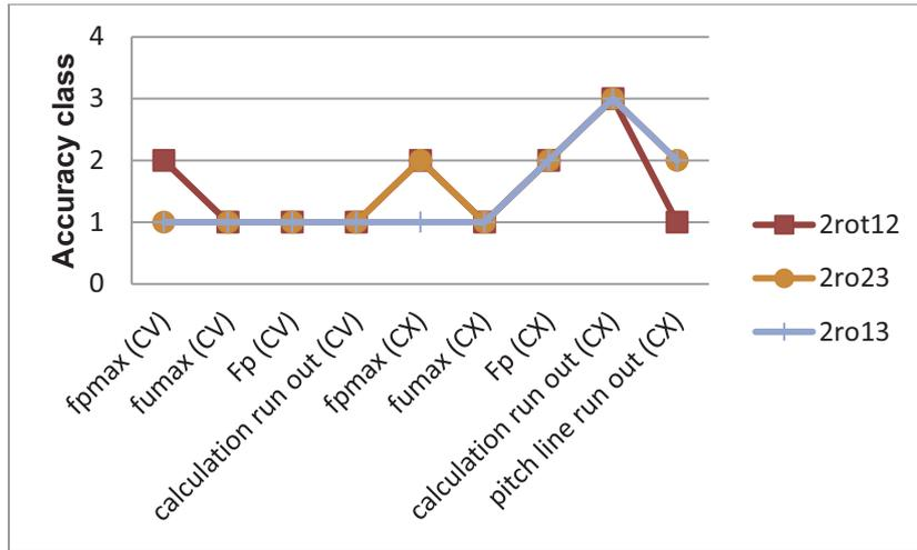
Fig. 9. Accuracy classes for individual parameters obtained from the measurement of a bevel pinion with circular pitch line for a fixation error compensation case based on 2 radial run-out measurements of the reference surface
