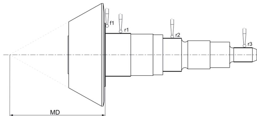
Fig. 2. Reference surfaces considered in the selection of object fixation compensation for the measurement
