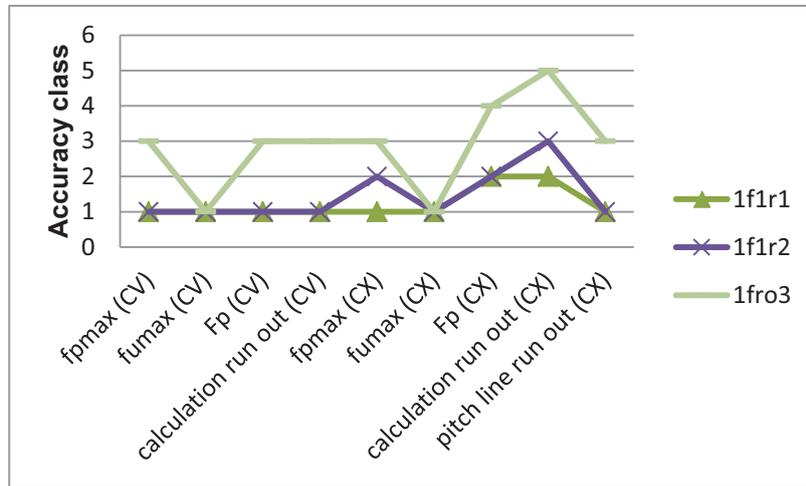
Fig. 10. Accuracy classes for individual parameters obtained from the measurement of a bevel pinion with circular pitch line for a fixation error compensation case based on 1 axial run-out measurement and 1 radial run-out measurement of the reference surface
