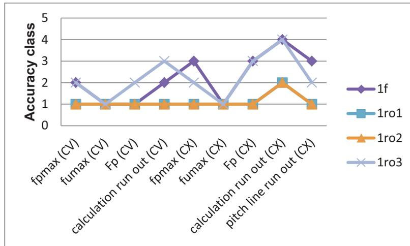
Fig. 11. Accuracy classes for individual parameters obtained from the measurement of a bevel pinion with circular pitch line for a fixation error compensation case based on 1 axial run-out measurement or 1 radial run-out measurement of the reference surface
