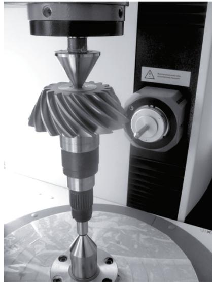
Fig. 1. A bevel pinion in the P40 machine's measurement space
