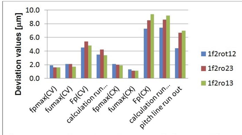
Fig. 3. Performance deviation values (*fpmax*, *fumax*, *Fp*, run out calculation, pitch line run-out) obtained from the measurement of a bevel gear with circular pitch line, whose fixation error compensation is based on 1 axial run-out measurement and 2 radial run-out measurements of the reference surface
