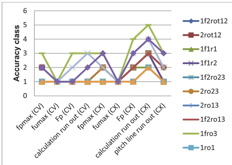
Fig. 7. Summary list of accuracy classes for individual parameters obtained from the measurement of a bevel pinion with circular pitch line for individual cases of fixation error compensation
