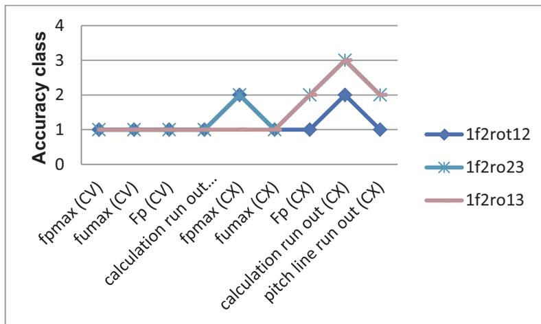
Fig. 8. Accuracy classes for individual parameters obtained from the measurement of a bevel pinion with circular pitch line for a fixation error compensation case based on 1 axial run-out measurement and 2 radial run-out measurements of the reference surface
