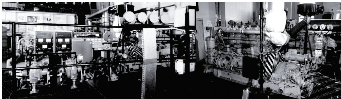
Fig. 1. WOLA engine type 57H6Aa test stand with hydraulic brakes
