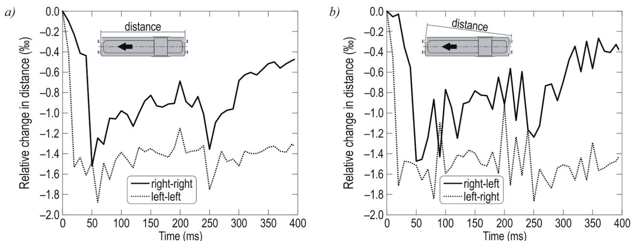
Fig. 9. Relative changes in longitudinal (a) and diagonal (b) distance between buffer attachments
