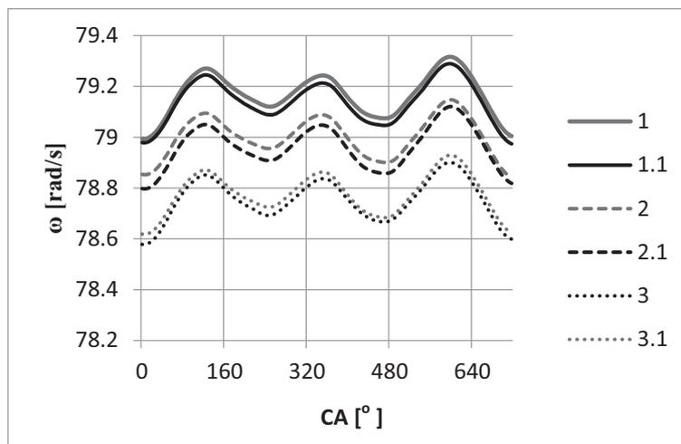
Fig. 1. Angular speed of healthy engine recorded in three different atmospheric conditions
