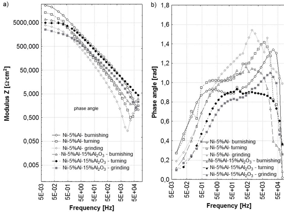
Fig. 5. Examples of Body plots: a) modulus of impedance and b) phase angle for the flame sprayed by Casto-Dyn DS 8000 torch Ni – 5% Al and Ni – 5% Al – 15% Al<sub>2</sub>O<sub>3</sub> coatings, after finishing treatment [10]
