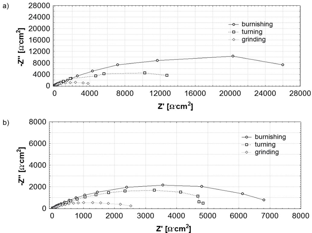
Fig. 4. Examples of Nyquist plots for the flame sprayed by Casto-Dyn DS 8000 torch a) Ni – 5% Al b) Ni – 5% Al – 15% Al<sub>2</sub>O<sub>3</sub> coatings, after finishing treatment
