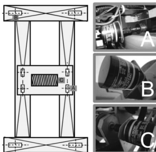
Fig. 1. The rotary encoders mounted on the scaled laboratory model of the overhead travelling crane
