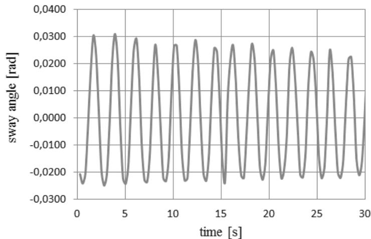
Fig. 7. Free sway rope measured with the vision system
