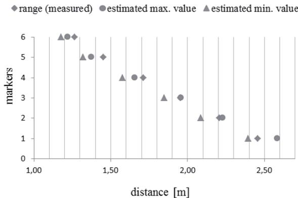
Fig. 5. Summary of results obtain from the one camera stereovision system – perspective uncertainty range visualization
