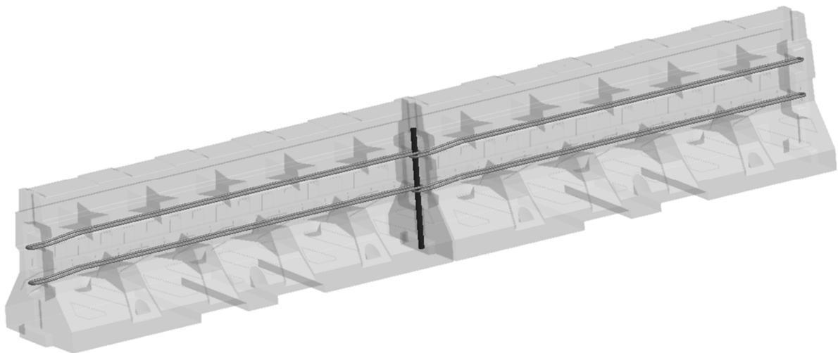
*Fig.2. Safety barrier segment connecting method*
