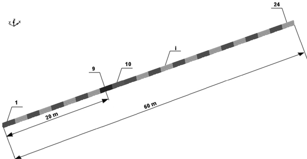
Fig. 5. Barrier configuration using two deformable segments (9 and 10):  $i$  – segment number
