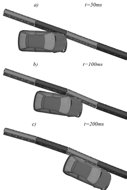
Fig. 7. Stages of a collision of the car and the barrier: a) for  $t = 50$  ms, b) for  $t = 100$  ms, c) for  $t = 200$  ms
