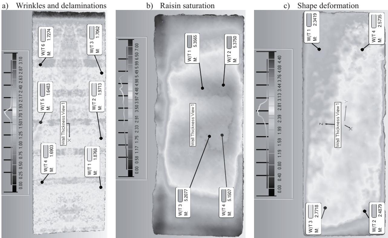
Fig. 3. Vacuum technology manufactured composite specimens – defects
