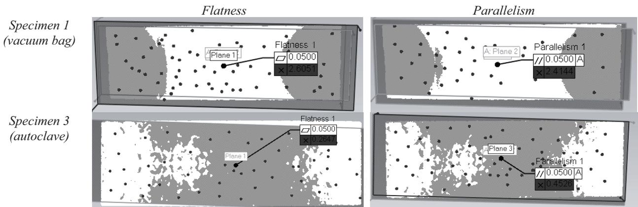
Fig. 5. Geometric dimension and tolerancing (GD&T) – selected specimens
