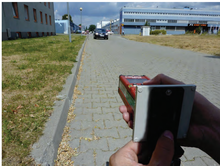
Fig. 2. Measurement of standard distance between photo barriers
