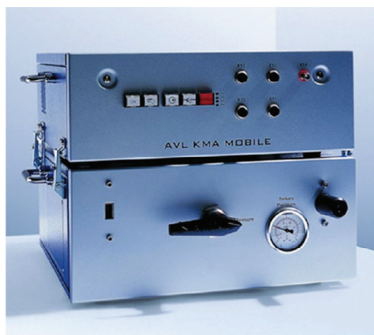
Fig. 2. The AVL KMA Mobile flow meter with fuel conditioning system [5]
