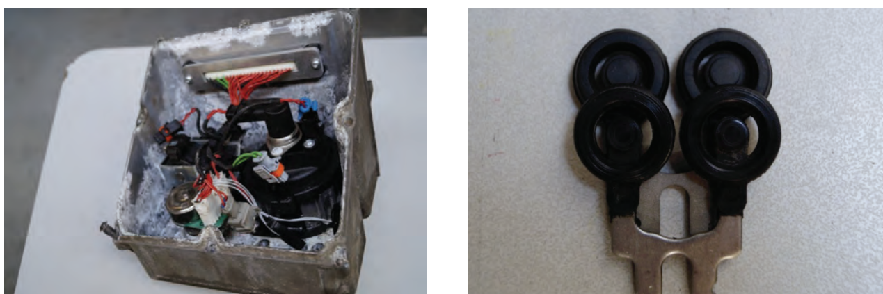
Fig. 5. View of ad-blue agent leakage inside the pump enclosure (left), and application of e.g. fuel oil instead of ad-blue agent results in many designs in immediate damage of pump's rubber components (right) (Piotr Stryjek)
