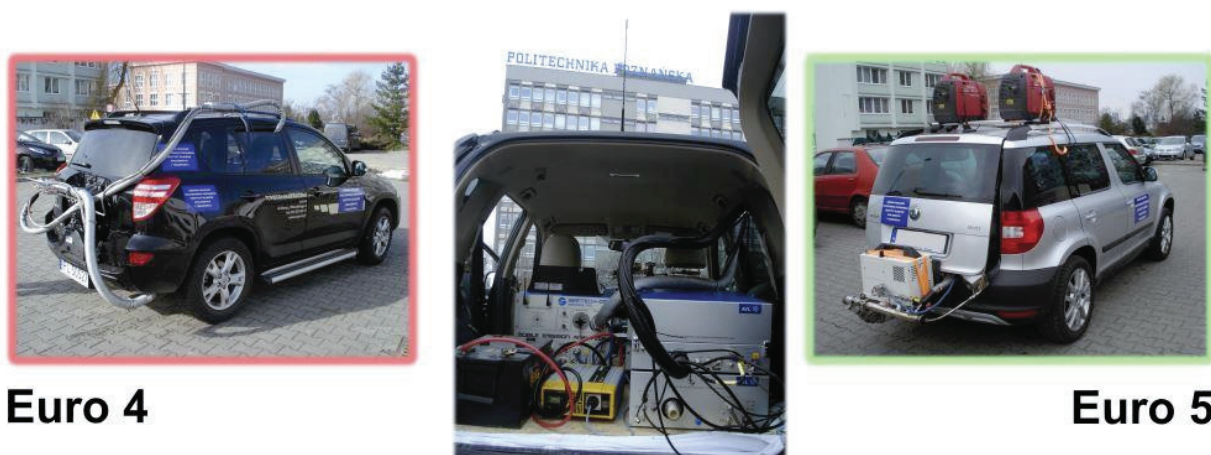
Fig. 2. View of the portable exhaust emission measurement system (SEMTECH DS)
