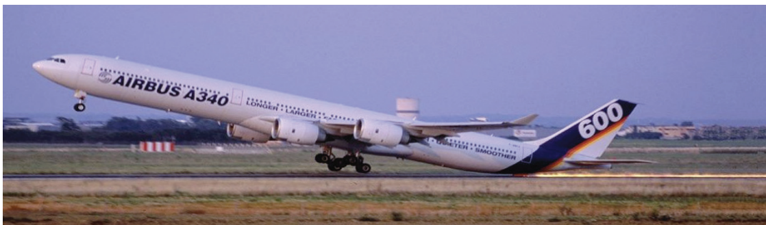
Fig. 3. Airbus A340 at the detachment at a minimum velocity separation [6]
