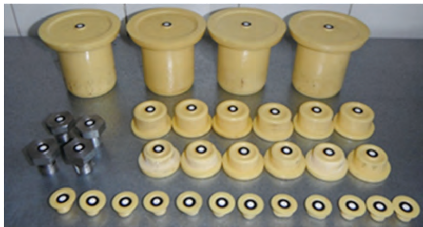
Fig. 4. Test adapters printed in 3D technology
