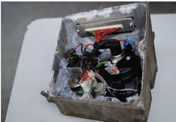
Fig. 5. View of ad-blue agent leakage inside the pump enclosure (left), and application of e.g. fuel oil instead of ad-blue agent results in many designs in immediate damage of pump's rubber components (right) (Piotr Stryjek)
