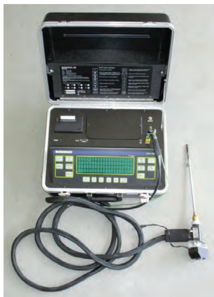
Fig. 10. ECA 450 combustion efficiency analyser
