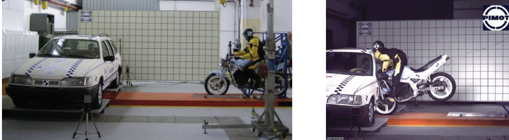
Fig. 1. Positions of the vehicles prior to the collision and at t = 100 ms
