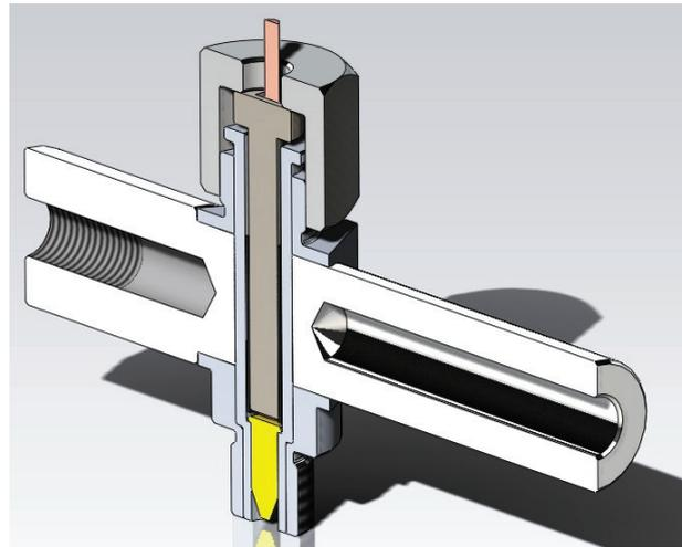
Fig. 3. Blank Ammunition Initiator
