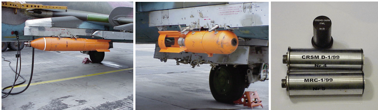
Fig. 3. Data recorders for flight parameters installed on avionic bombs with standard weight of 250 and 50 kg
