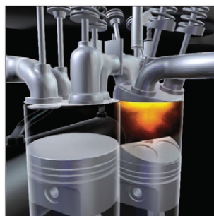
Fig. 1. Scuderi engine (on the left compression cylinder) [12]
