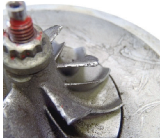
Fig. 13. View of compression rotor with tracks caused by small body
