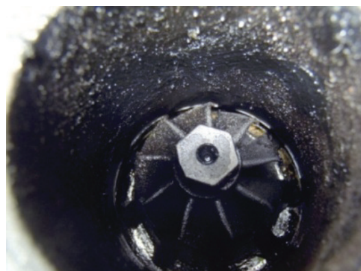
Fig. 10. View of turbine rotor with carbon depositing
