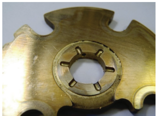
Fig. 3. View of scraped surface of bearing
