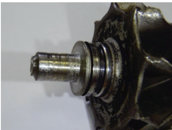
Fig. 2. View of broken rotor’s shaft necks with deep scrapes
