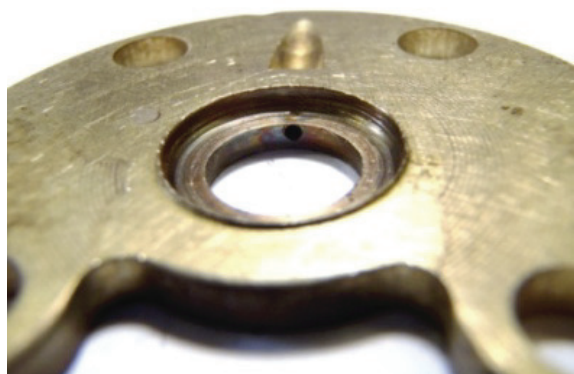
Fig. 11. View of bearing with hot tracks
