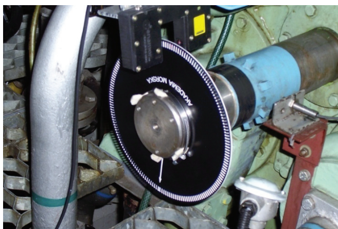
Fig. 1. Perforated disc and laser sensor mounted at crankshaft's free end
