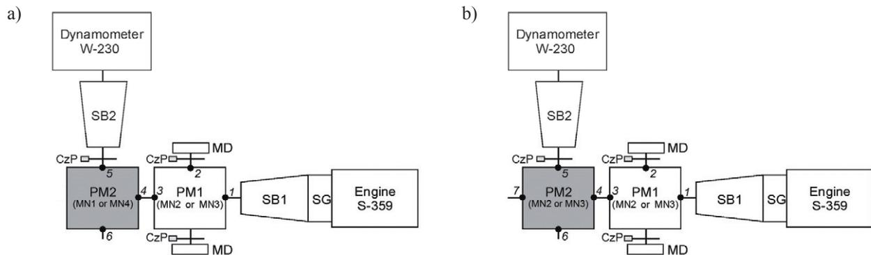
Fig. 1. Arrangement of measurement points: a) configuration of tested gear positions including central gear (PM1) and external (PM2), b) configuration of tested gear positions including the two central gear (PM1 and PM2)
