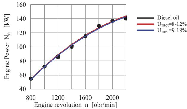
Fig. 4. Comparison of maximal power output of the SW 680 engine run in dual fuel system – fuelled with Diesel oil and methanol
