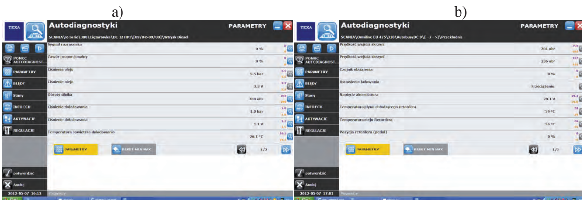
Fig. 5. TEXA Windows presented powertrain work parameters: a) SCANIA engine, b) ZF gear box (Source: by authors)
