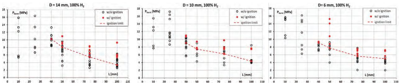
Fig. 7. Cumulative diagrams for pure hydrogen flow through tube with  $d = 14, 10$  and  $6 \text{ mm}$  and various tube lengths
