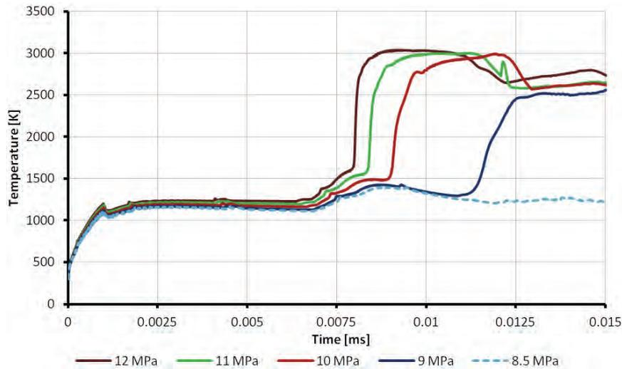
Fig. 5. Calculated temperature in subsequent cases with ignition compared to no ignition case,  $L = 20 \text{ mm}$
