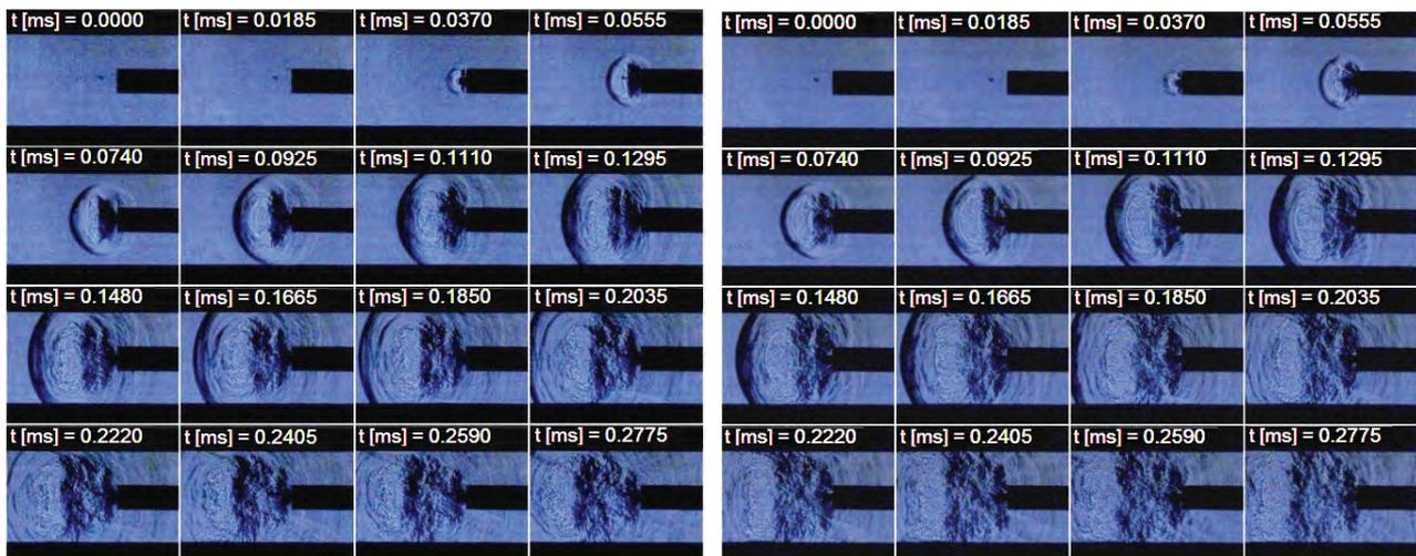
Fig. 9. Schlieren images (recording speed 54 000 fps, 1/297000 s shutter) for cases  $d = 6$  mm,  $L = 75$  mm, with ignition (left,  $P_{burst} = 7.15$  MPa) and without ignition (right,  $P_{burst} = 4.28$  MPa), time  $t = 0$  s specified arbitrarily
