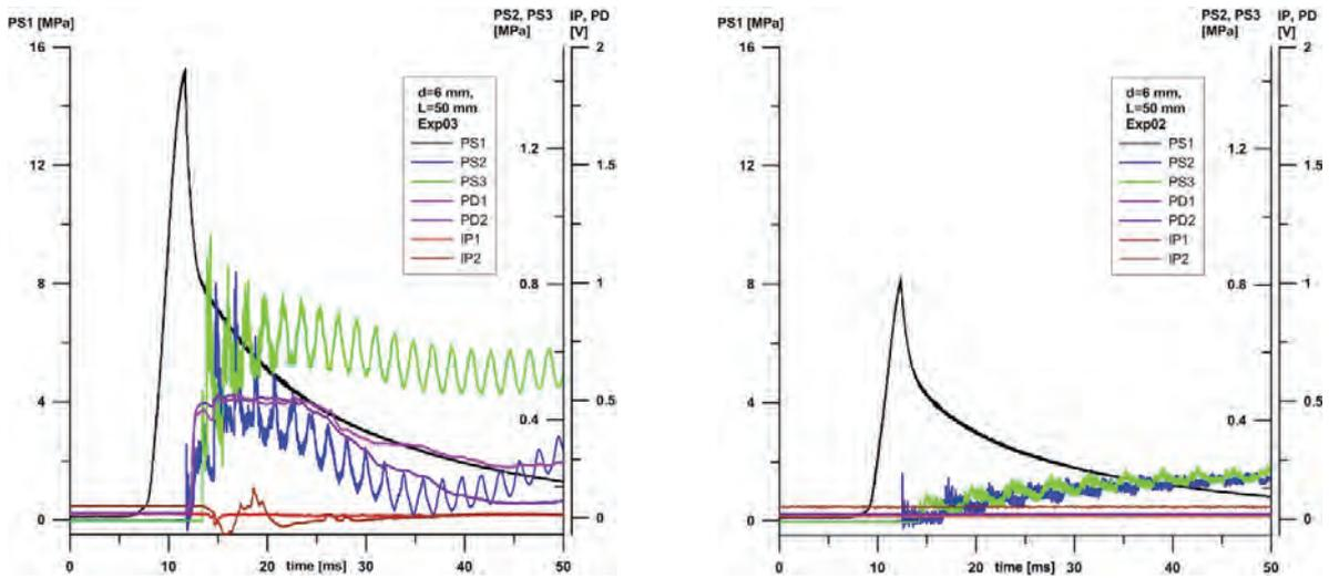
Fig. 6. Sensors indications for cases  $d = 6 \text{ mm}$ ,  $L = 50 \text{ mm}$  with ignition (left,  $P_{burst} = 15.3 \text{ MPa}$ ) and without ignition (right,  $P_{burst} = 8.4 \text{ MPa}$ )
