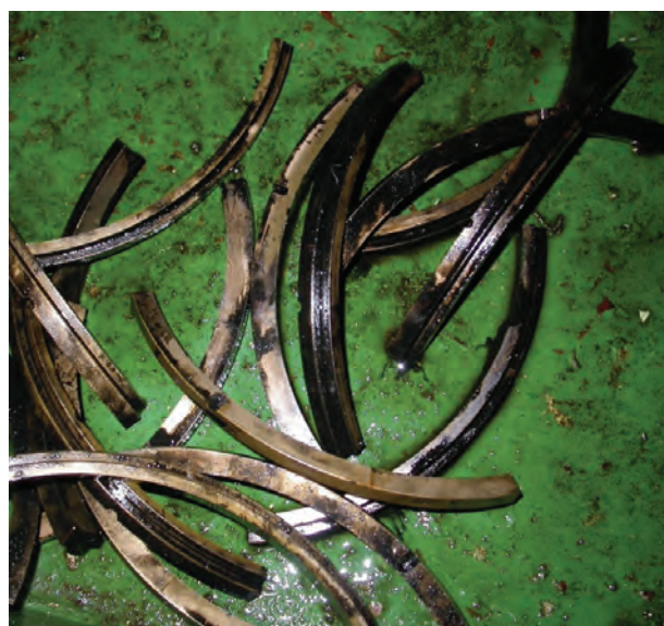
Fig. 6. Broken piston rings of main engine
