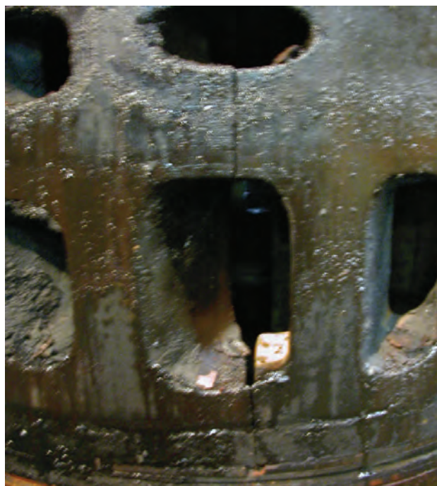
Fig. 5. View of cracked cylinder liner
