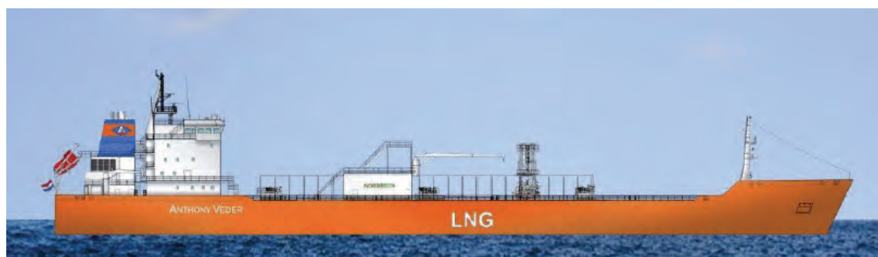
Fig. 6. 15600 m 3 LNG carrier (TGE-Marine design) – delivered December 2012 [13]
