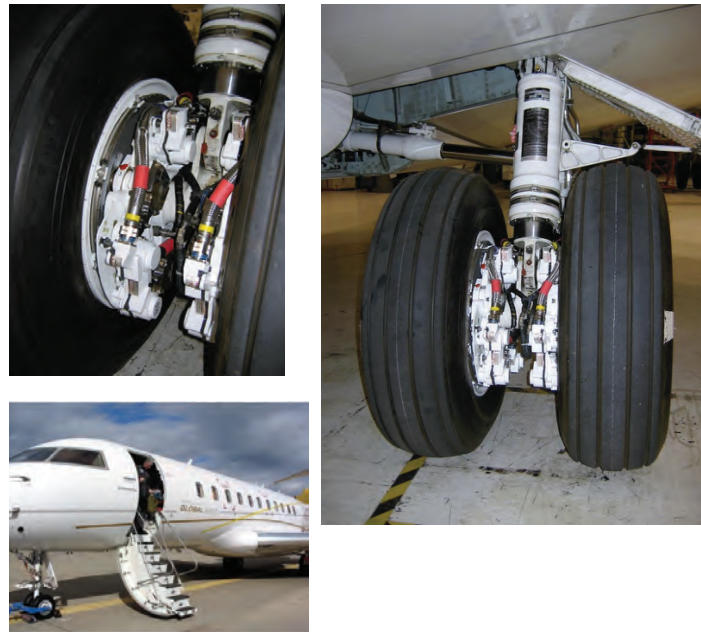
Fig. 2. The example of the Meggitt's Ebrake tested on Bombardier global 5000 [9]
