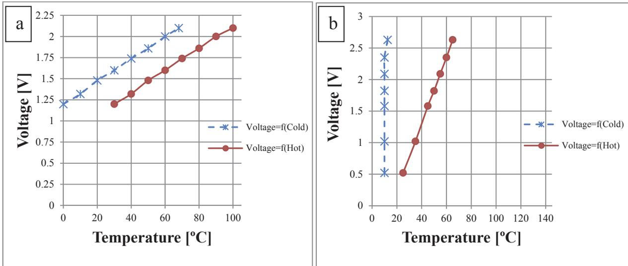
Fig. 4. Parameters of the surveyed TEG: a) for a constant temperature difference between the cold and hot side,  $\Delta T=30^{\circ}\text{C}$ , b) for a constant temperature of the cold side  $T_c=10^{\circ}\text{C}$  and an increasing temperature of the hot side
