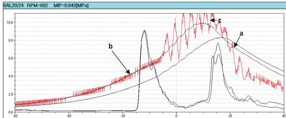
Fig. 6. An example of the pressure curve reconstruction: a – pressure curve measured without throttling, b - pressure curve measured with throttling of the channel, c - b pressure curve after reconstruction
