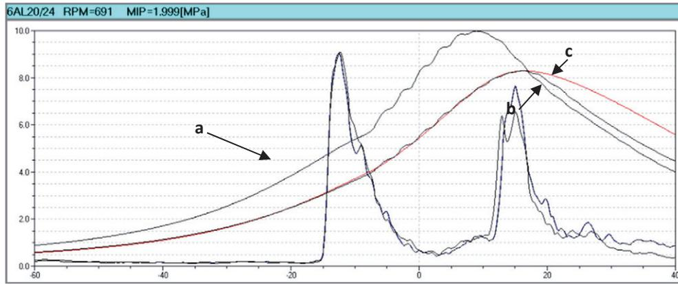
Fig. 5. Test of the IIR filter as a model of indicating channel choking: *a* – pressure course measured without throttling, *b* - pressure course measured with throttling of the channel, *c* - the course *a* after the filter with coefficient  $a = 0.0078$
