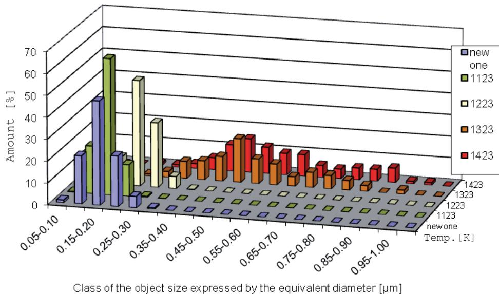
Fig. 7. Number of precipitations within individual size classes of  $\gamma'$  phase particles for the material of turbine blades, for a new blade and blades heated to the temperatures from 1123 K to 1523 K
