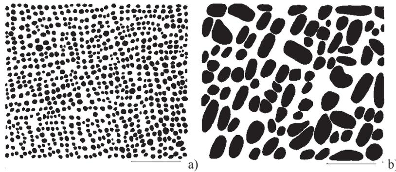
Fig. 6. The microstructure of turbine blades after heating at temperatures: a) - 1123 K, b) - 1423 K (magn. x20000) – one can see coagulation, alteration of shapes and corrugation of the  $\gamma'$  phase formations.
