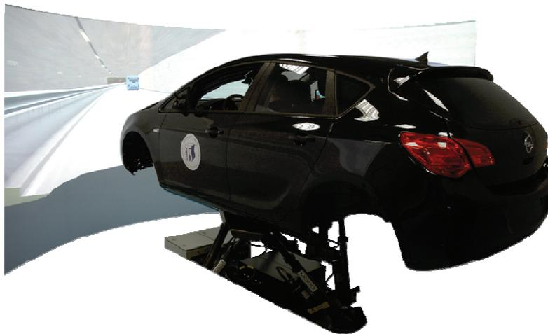
Fig. 2. AutoSim AS 1200-6 advanced high-class car simulator
