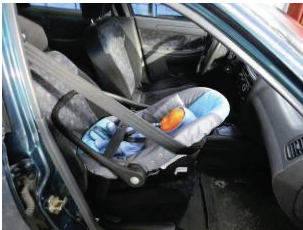
Fig. 4. Safety seat with the BABY dummy, installed on the front seat
