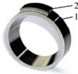
Fig. 1. The sliding pair: 1 – ring specimen, 2 – counterpart
